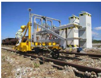
Figure 14. Test equipment of Ground penetrating radar [33]
