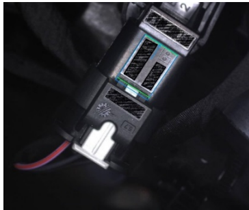
Figure 2. The measurement of the distance between upper edge of the plastic label and the connector lock
