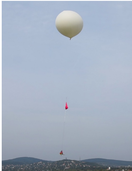
Figure 1. A light unmanned free balloon
