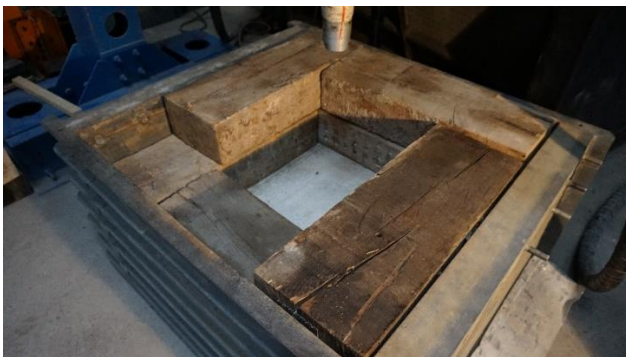
Figure 3. The wooden sleepers in the shear box
