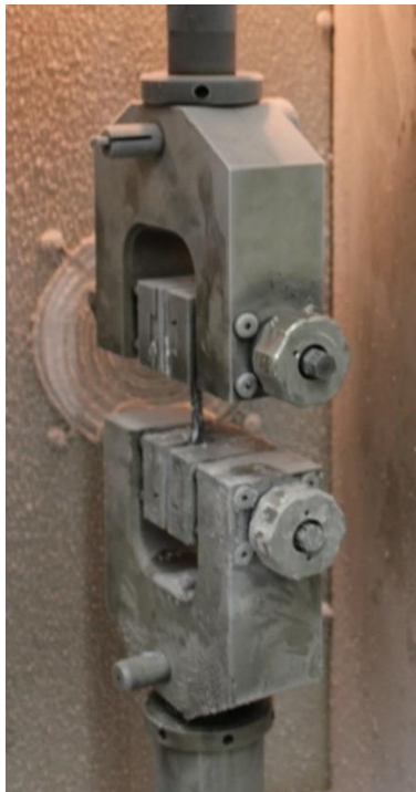
Figure 5. Standard test specimen at -40 °C, placed in climate chamber
