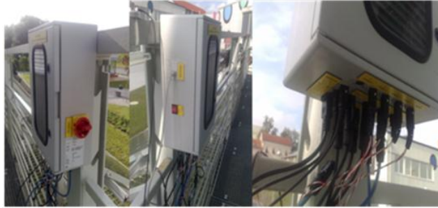
Figure 1. Measuring system for characteristics monitoring of PV modules (MSPV01)
