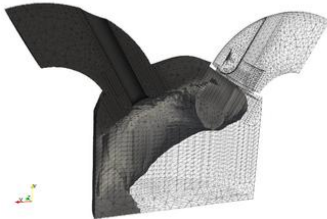
Figure 1. Combustion chamber during the intake phase. The intake valve is at the bottom position. The freshly drawn gas is depicted as the dark range, showing where its relative density reaches 50%. The outlet valve is closed, and the corresponding cells are rendered inactive, thus are invisible here.
