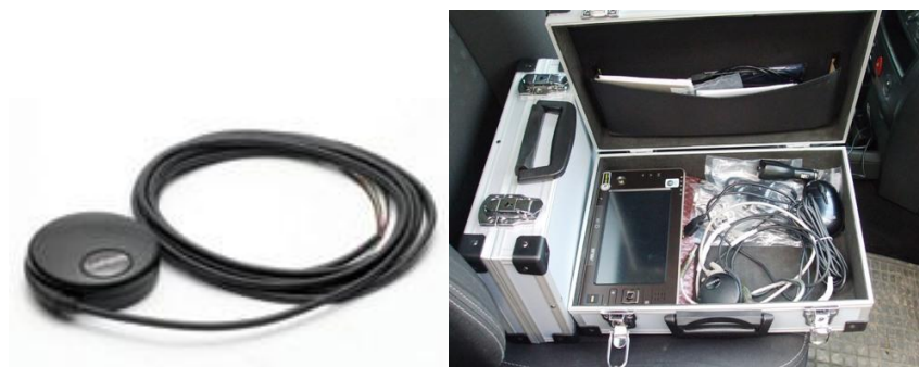
Figure 4. GPS 18x-5Hz and the DS-5 data acquisition system
