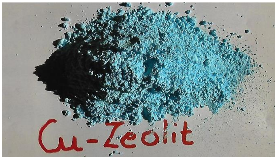
Figure 5.: Ion-exchanged zeolite with powdered copper-amine-complex ion, (self-photograph)
