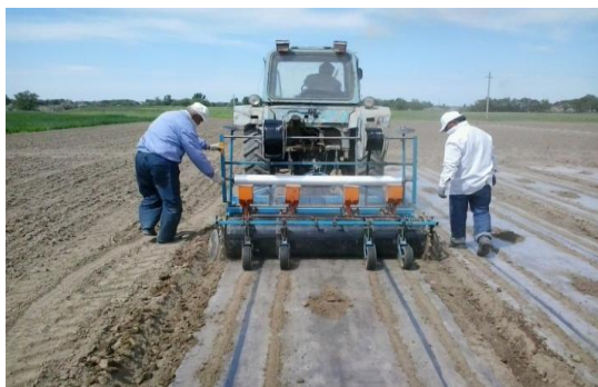
Figure 4. Double-row rice sowing with laying of both irrigation tape and tensioning of the film
