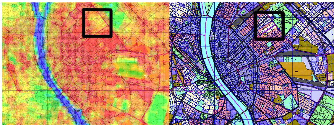
Figure 5. The role of the different built-up types: next to the City Park (towards the city centre) can be found a small cooler area represented by yellow color on the left infrared image, which can be exactly coupled with the detached built-up type area represented on the regulation plan (right). The infrared image was shot on 6 th July 2001.
