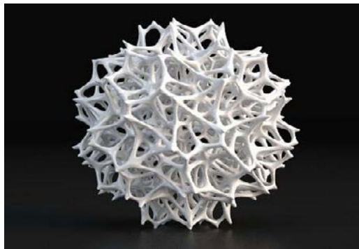
Figure 7 Complicated-shaped part produced by a 3D printer
