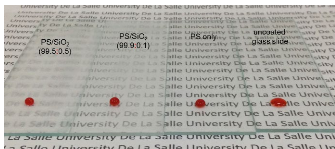
Fig. 4. PS films incorporated with different amounts of Aerosil R816 (PS/AS3) applied on glass compared to just bare PS coating and uncoated glass slide
