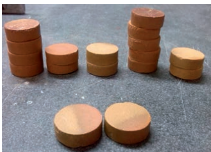
Fig. 4. The sintered at 1250°C ceramic disc specimens with different volumes of Al 2 O 3 and ZrO 2 powders in the raw material mixtures
