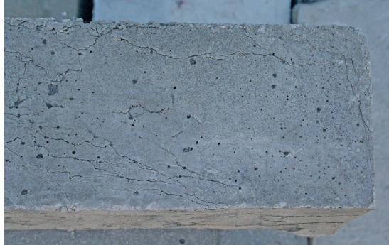
Fig. 3. Damaged specimen after 10 freeze-thaw cycles
