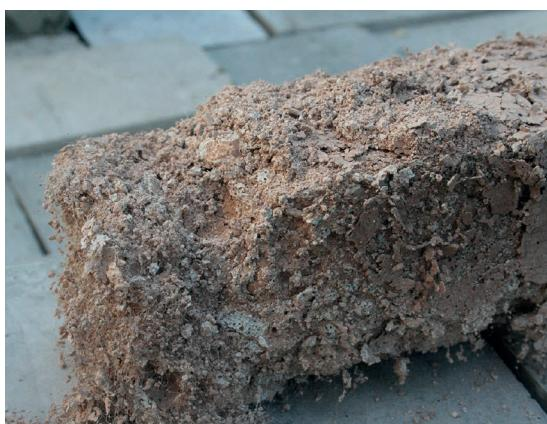
Fig. 4. Damaged specimen after 25 freeze-thaw cycles
