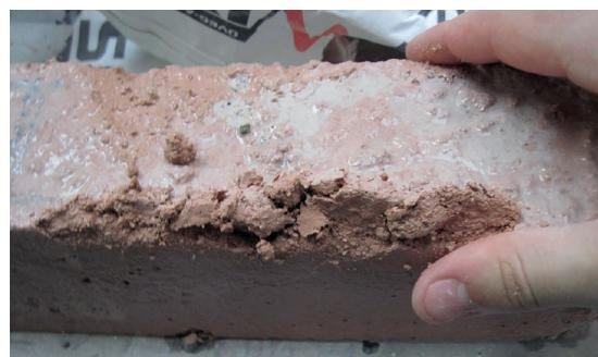
Fig. 5. White cement mixtures peeling in hand
