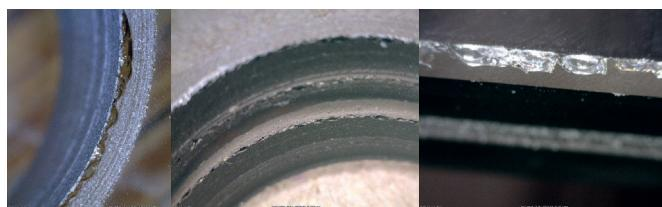
Fig. 4 Bore holes and edge defects at 50x magnification.
