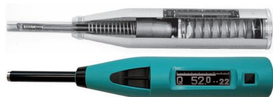
Fig. 1. Original Schmidt rebound hammer and Silver Schmidt rebound hammer
