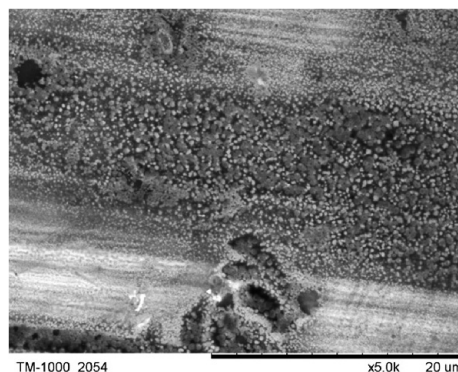
Fig. 4. Typical defects on surface of copper filaments
