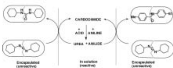
Figure 6. The reaction cycle that leads to autocatalytic behavior. Free carbodiimide generates two products, the urea and anilide. Each of these is capable of displacing carbodiimide from the capsule and increases the concentration of DCC, free in solution.
