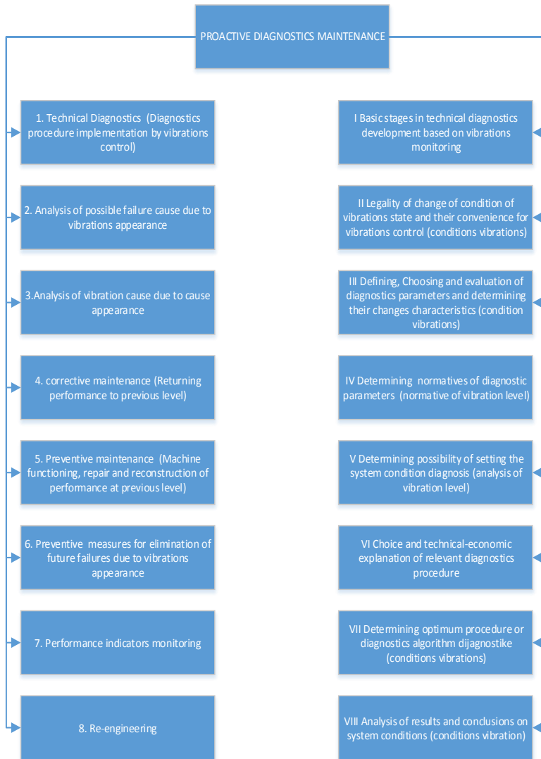
Figure 3 Model of proactive diagnostic maintenance
