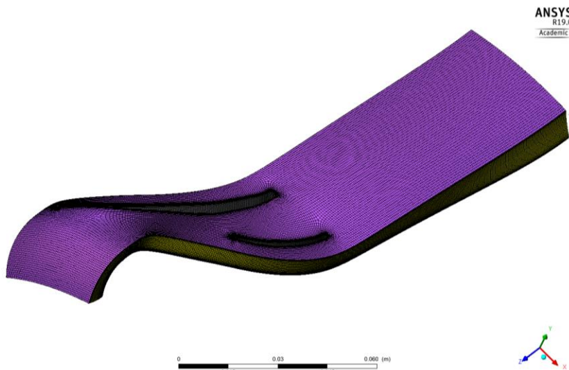
Figure 4 Computational mesh of the stator
