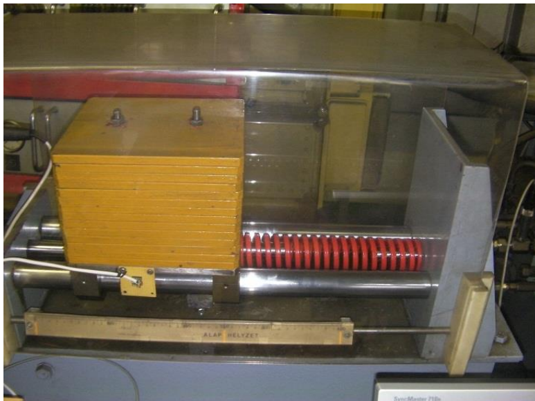
Figure 10 Mass-spring mechanical load of the positioning system
