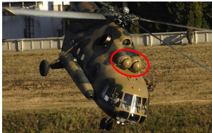
Fig. 5. PZU dust separator on Mi-17 transport helicopter
