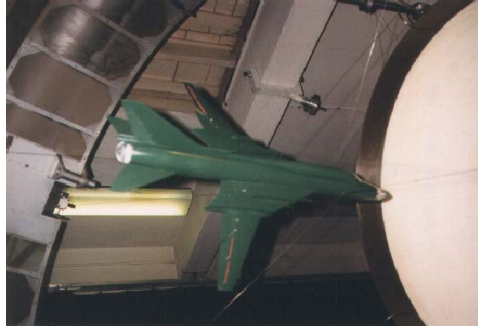
Fig.6. Aircraft model with the sweep angle \chi_{sk} = 30^\circ in the wind tunnel
