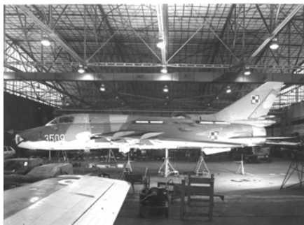
Fig.1. Aircraft Su-22 set up to determine the co-ordinates x , y , z
