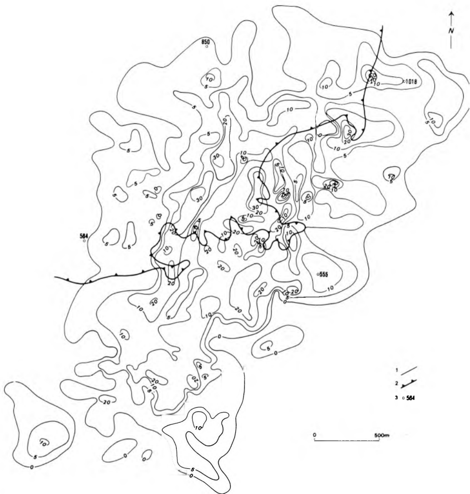
Fig. 25. Isopach map of the Halimba Bauxite Deposit based on the map of F. SZANTNER (1966)
