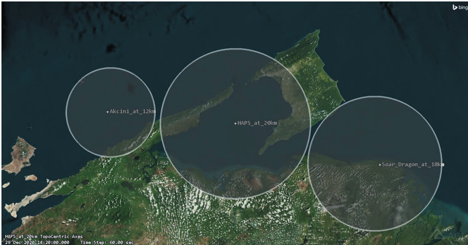
Figure 8: Overhead visualisation of the coverage areas of a HAPS and two HALE RPAS
