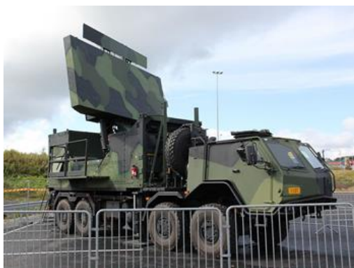
Figure 10. Ground Master 403 radar [21]
