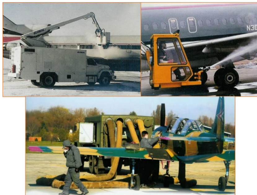
Figure 17. Chemical defrosters and hot air engines [35].
