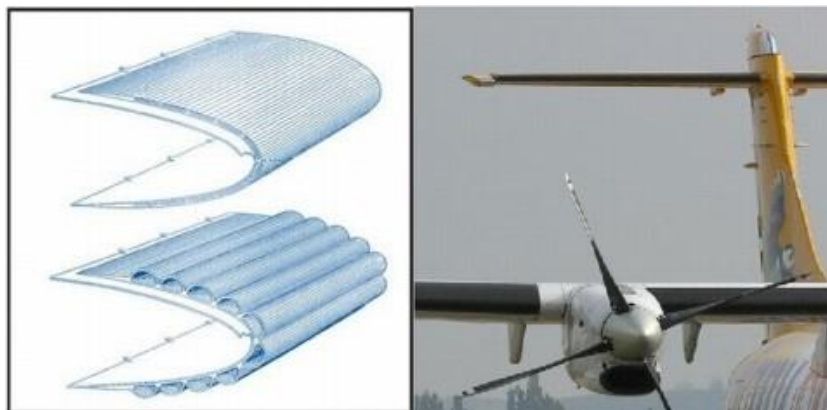
Figure 14. Pneumatic de-icing system [35]
