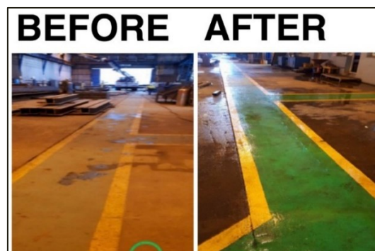
Figure 6.: Implementing of 5s in the pathway(Safety)
