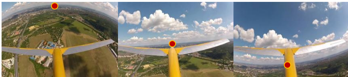
Figure 7. Movement of the horizon on the image plane as perceived by the wide angle lens video camera
