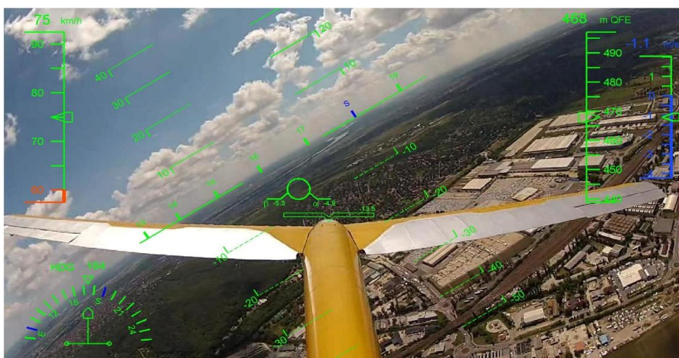
Figure 13. Screenshot of HUD projected on the wide angle lens camera recording
