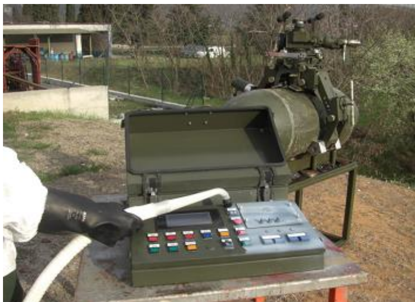
2. Figure. The CRISTANINI sensitive equipment detoxification SX34 decon vacuum in use. [6]
