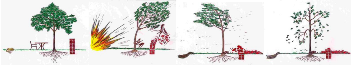
Figure 3. Blast wave mechanism [9]
