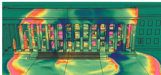
Figure 6. Blast loads on a building frontage [11]
