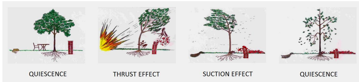
Figure 10: Impacts caused by explosion [6]
