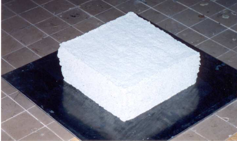
Figure 4. Single-layer paper fibre mat
