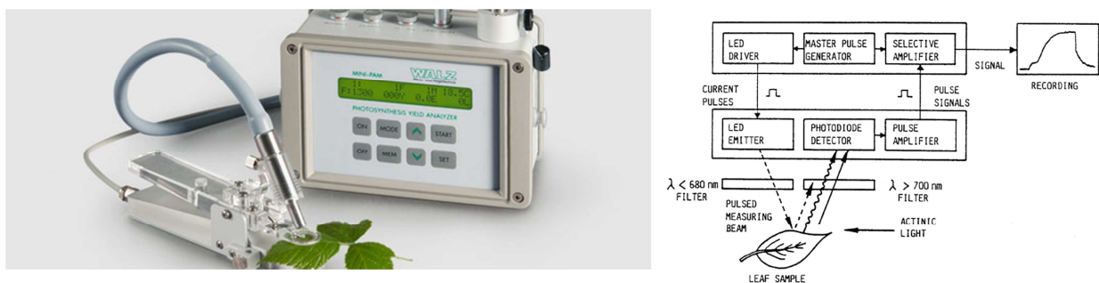
Figure 4: MINI-PAM Photosynthesis yield analyzer and the schematic view of the PAM measuring principle (source: http://www.odt.com.tw/ )
