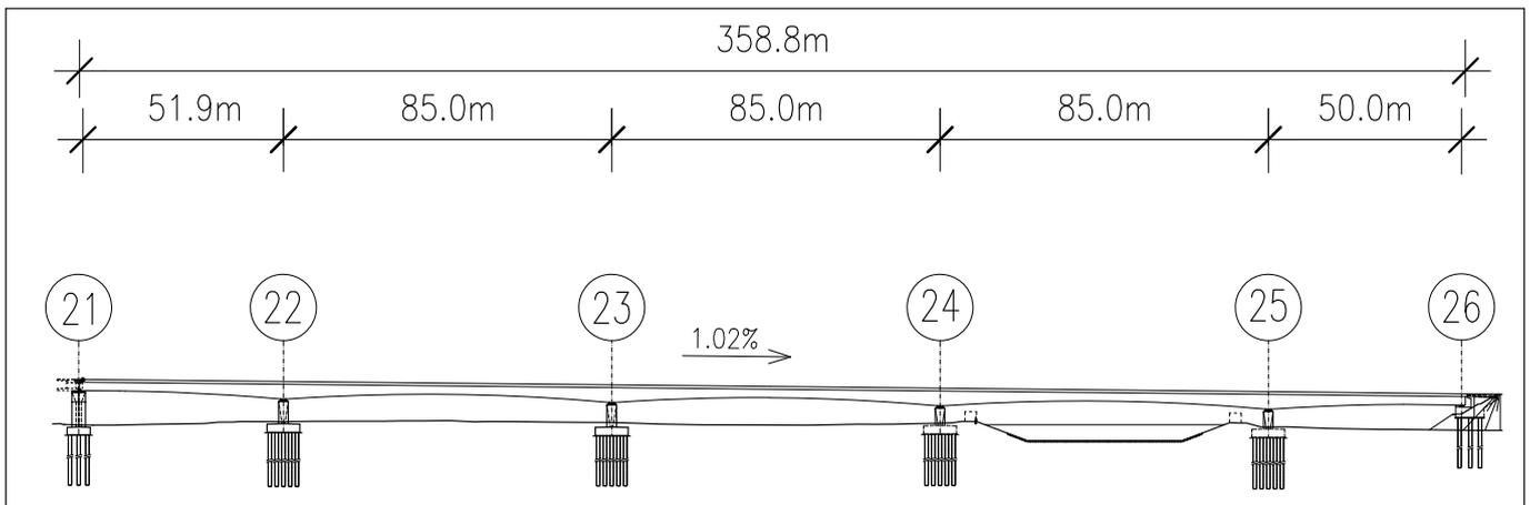
Fig. 3: Side view of the second dilatation unit (DC2)
