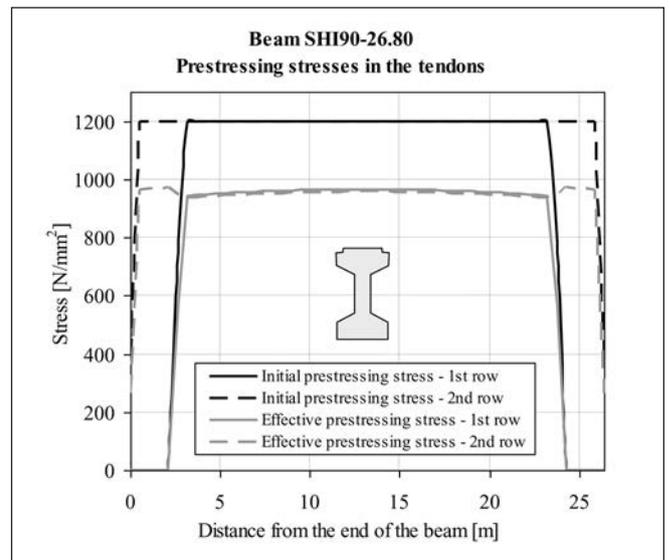
Fig. 2: Initial and effective prestressing stresses
