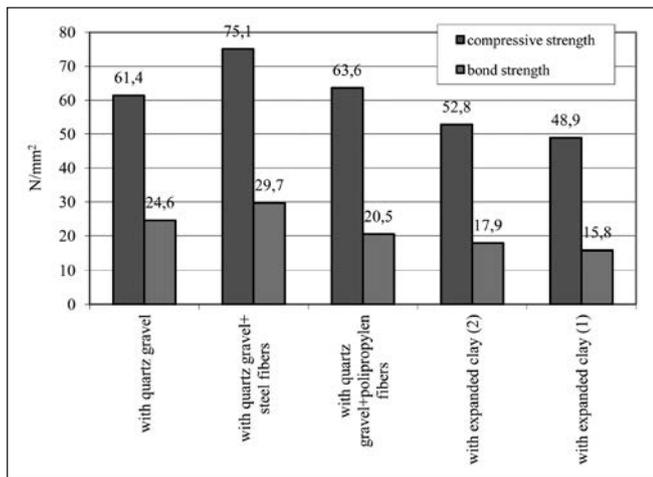
**Fig. 23:** Concrete compressive strength and bond strength with various mixes at 20°C
