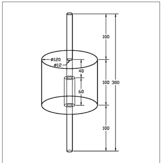
Fig. 22: Pull-out specimen
