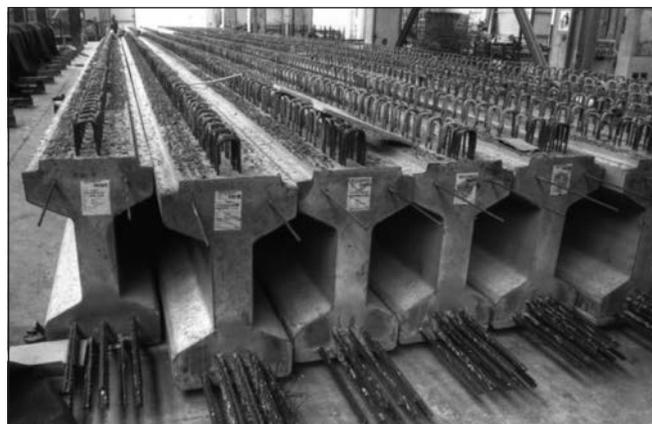
**Fig. 11:** Manufactured SHI90 beams at Majosháza site
