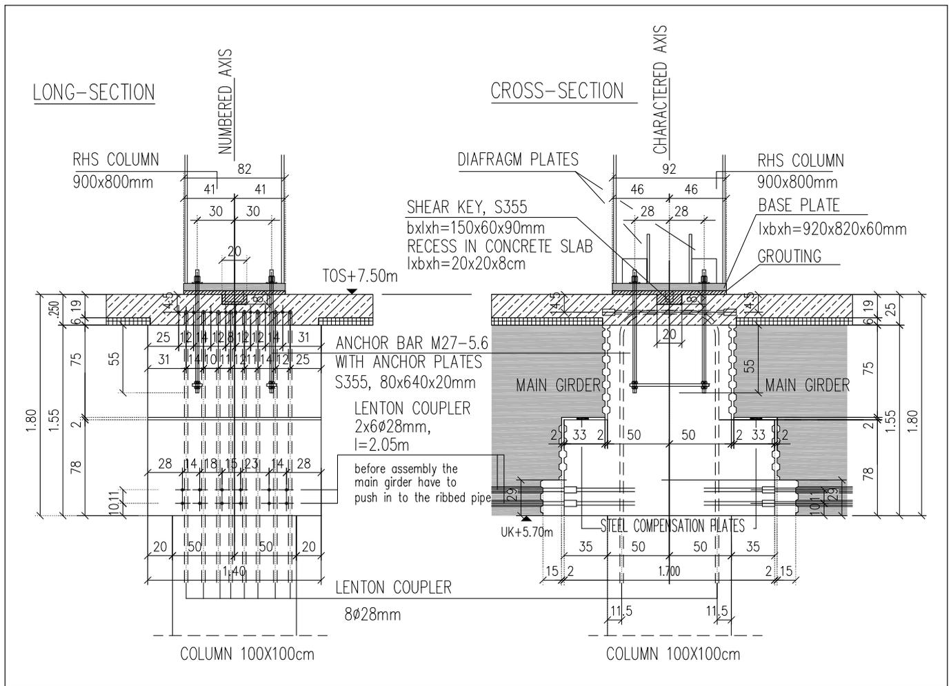
Fig. 4: Column-main girder rigid connection detail (detail from tender document)
