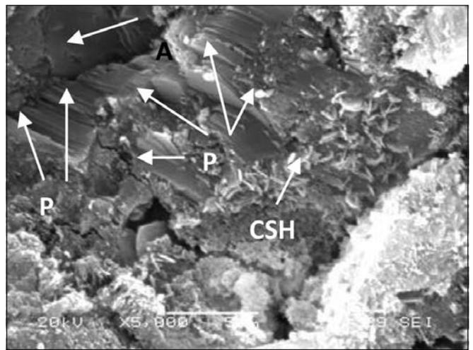
Fig. 6: N 5000 (SEM) Concrete using Portland cement
