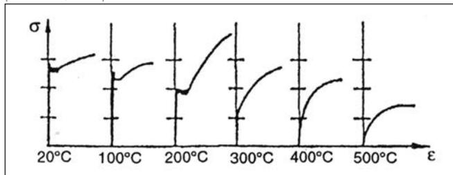
**Fig. 15:** Tensile strength of steel as a function of temperature (Felicetti, Meda, 2005)
