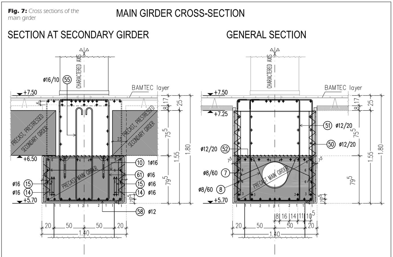
Fig. 7: Cross sections of the main girder
