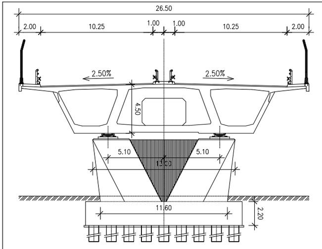
Fig. 4: Cross section of the second dilatation unit (DC2)
