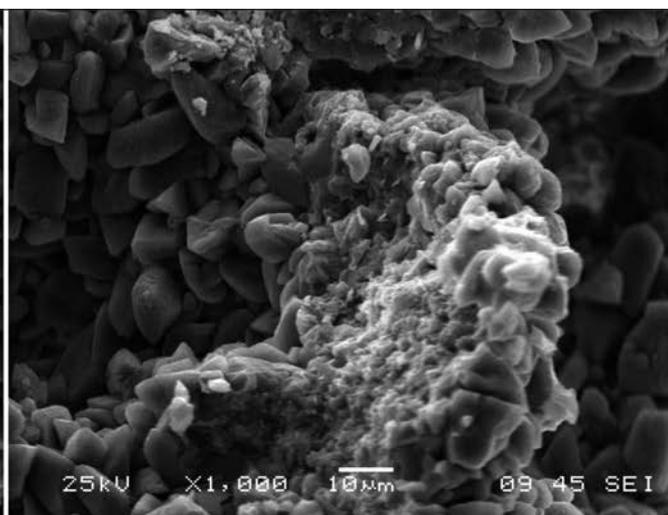
**Fig. 5.b:** Surface of the sample with small, spot-like groups of crystals at 1000X magnification
