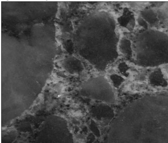
**Fig. 10:** Concrete with expanded clay aggregate at temperature of 20°C
