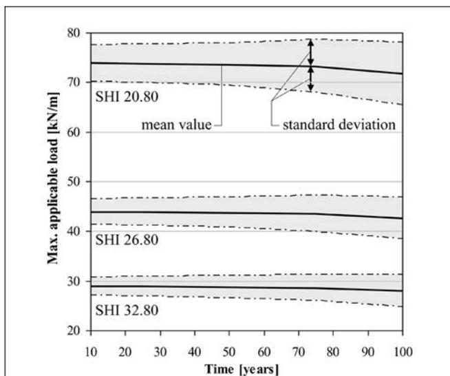
**Fig. 8:** Change of the mean value and standard deviation of load carrying capacity in case of different SHI120 beams
