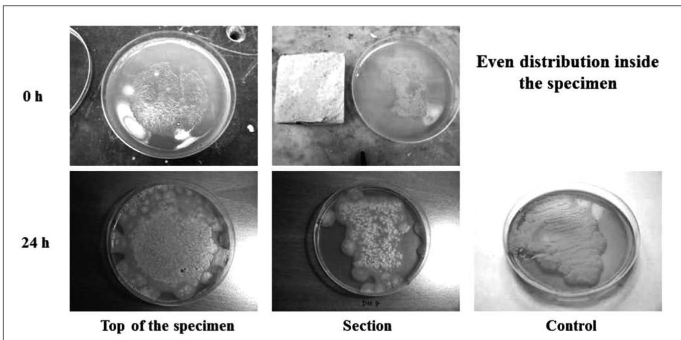
**Fig. 6:** Indirect evaluation of the effective penetration depth. Prints at 0 h and after 24 hours of incubation, and the control.
