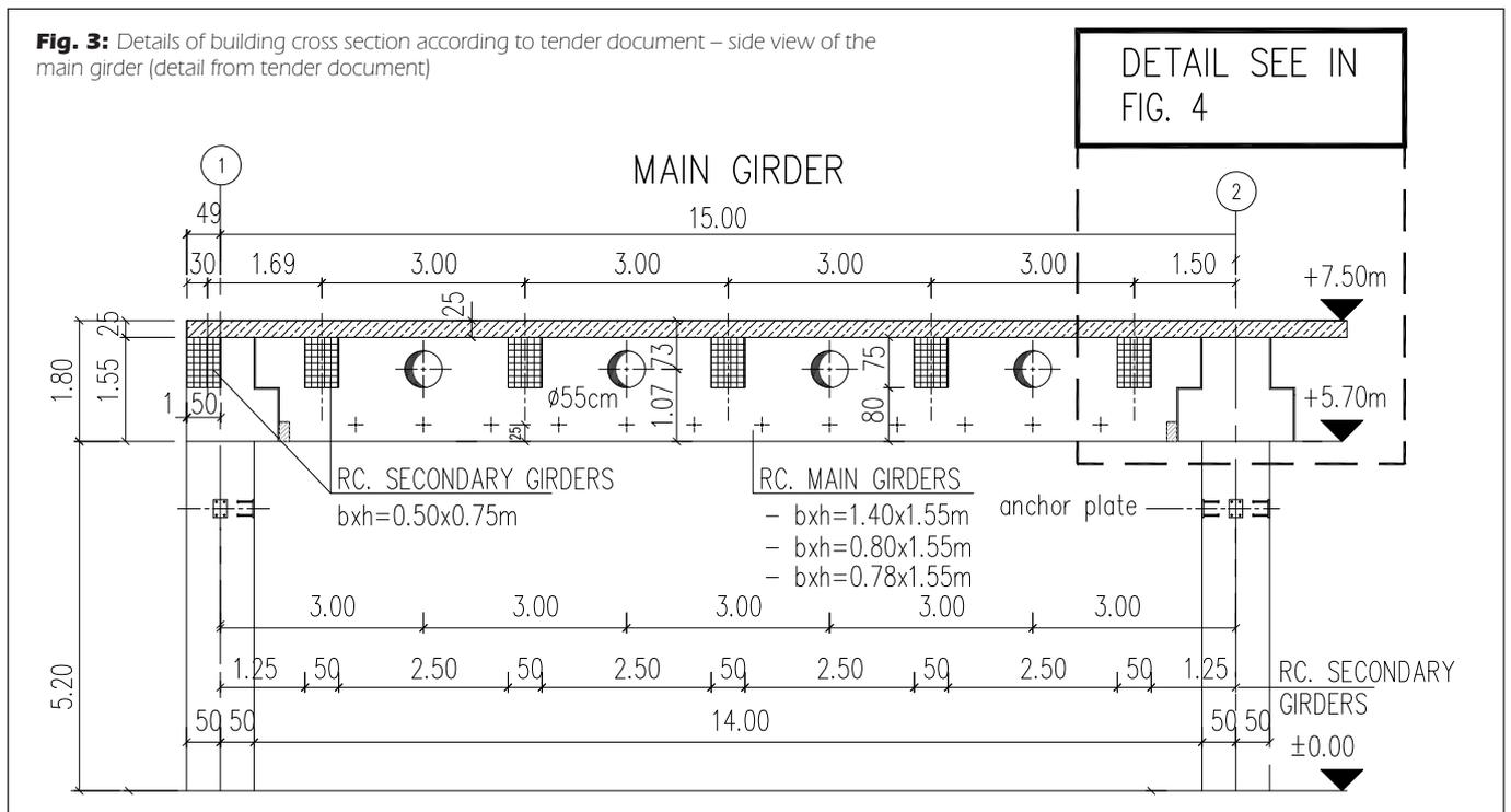
**Fig. 3:** Details of building cross section according to tender document – side view of the main girder (detail from tender document)
