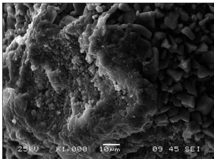
**Fig. 5.a:** Surface of the sample: original surface on the right, precipitation on the left at 1000 X magnification.
