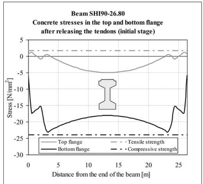
Fig. 3: Concrete stresses in initial stage
