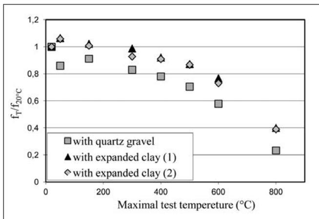
**Fig. 8:** Change of compressive strength after exposing the concrete to high temperature, measured at room temperature (20°C)
