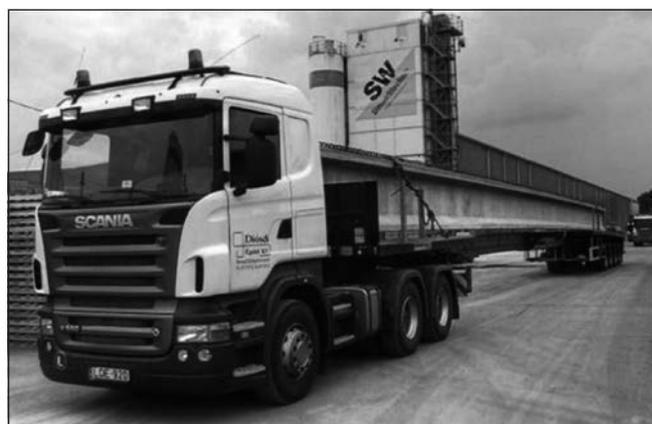
**Fig. 13:** Transportation of an SHI bridge girder
