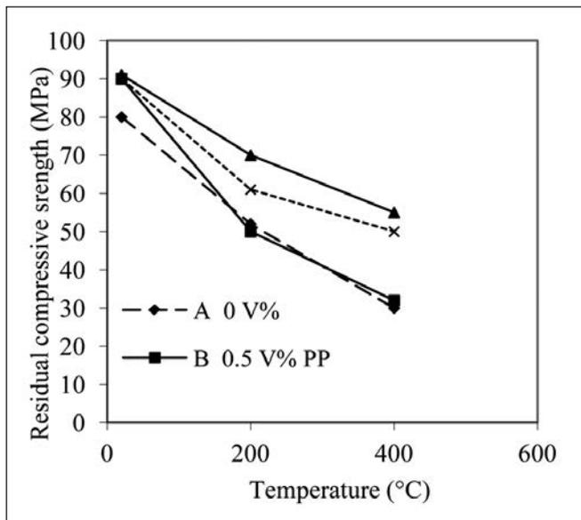
Fig. 19: Residual compressive strength of high strength concrete with or without fibres (Horiguchi, 2005)
