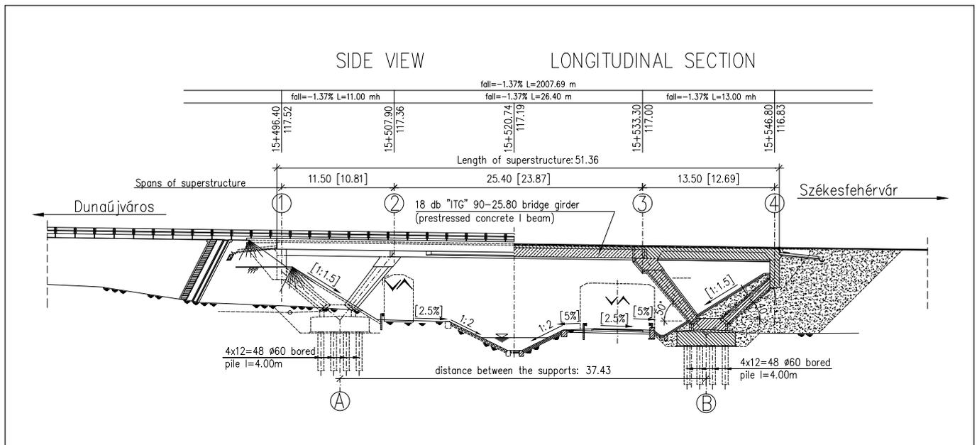
Fig. 16: Side view and longitudinal section of the Perkáta bridge
