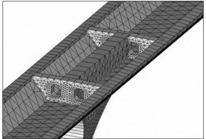
**Fig. 13:** The part of the M31 bridge deck underneath, above the internal leg. (from the finite element software)
