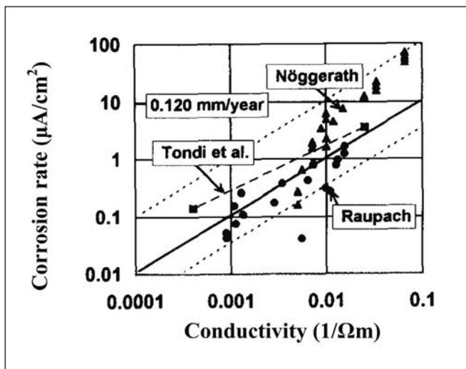
**Fig 6:** Corrosion rate as a function of the conductivity of concrete or mortar (Hunkeler, 1993)
