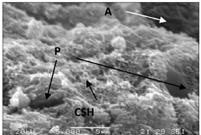
Fig. 7: N 5000 (SEM) Concrete using slag Portland cement
