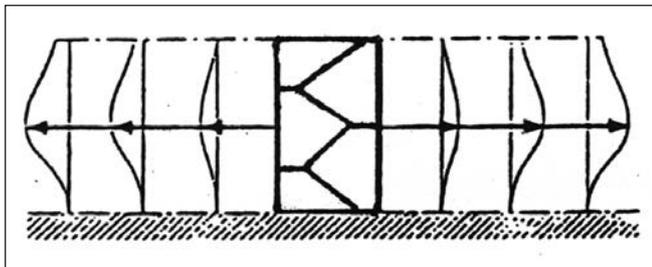
Fig. 20: Deformations during fire (fib, 2007)
