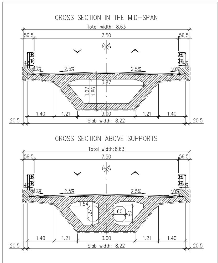
Fig. 11: Cross-section of the M31 bridge
