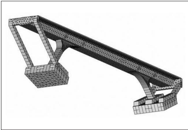
**Fig. 12:** The model of the M31 bridge in 3D by the Finite element software
