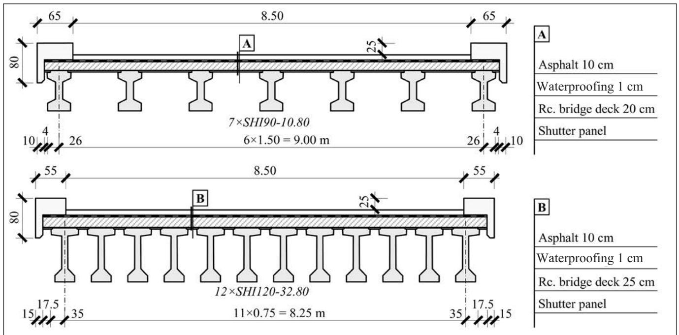
Fig. 5: Sample cross-sections of bridge superstructures consisting of SHI90 and SHI120 beams
