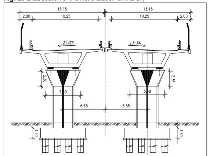
**Fig. 1:** Side view of the first dilatation unit (DC1)
