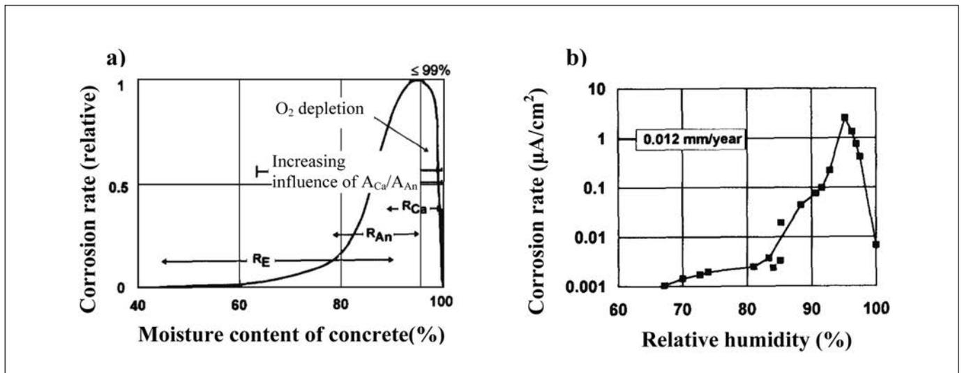
**Fig. 5:** a) Dependence of the corrosion rate on the water saturation and the influence of the different resistances ( $R_{An}$ : electrochemical resistance of the anode,  $R_{Ca}$ : electrochemical resistance of the cathode,  $R_E$ : electrolyte resistance of the concrete/mortar,  $A_{An}$ : area of the anode,  $A_{Ca}$ : area of the cathode) b) Corrosion of steel in carbonated mortar (Parrott, 1990)
