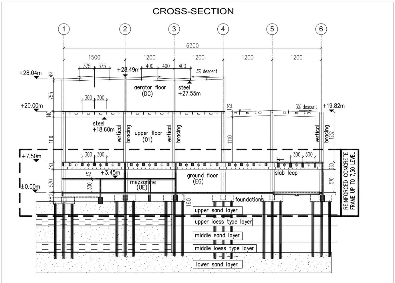
**Fig. 2:** Cross section of the building - schema of the structural frame (detail from tender document)
