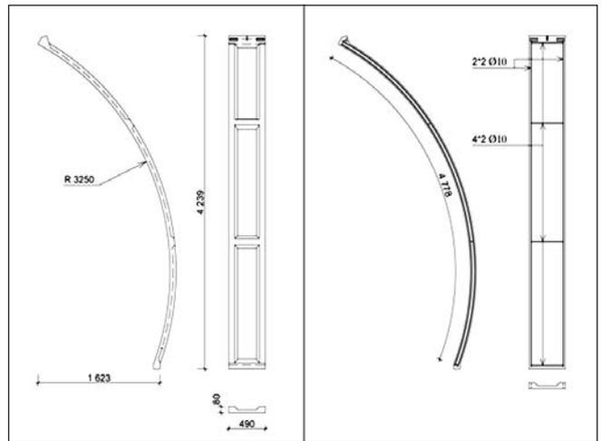
Fig. 6: Plan of the formwork and of the reinforcement for the station of the Fővám-square
