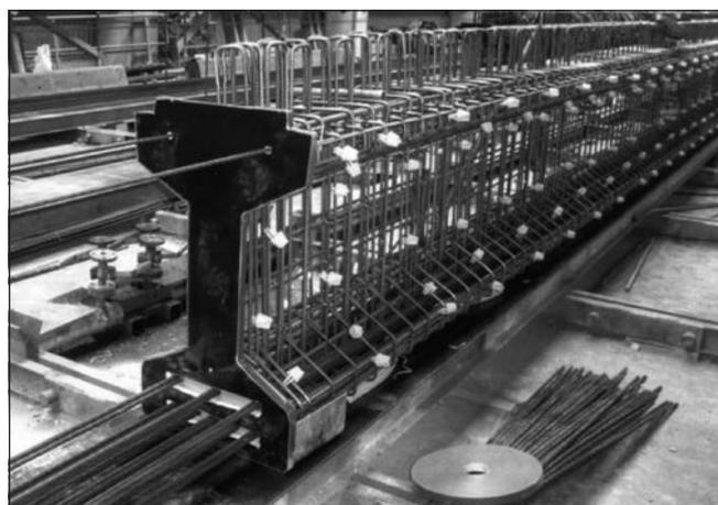
**Fig. 10:** Reinforcement of the SHI90 beams
