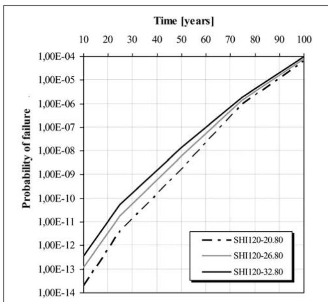
**Fig. 9:** Change of the probability of failure in case of different SHI120 beams
