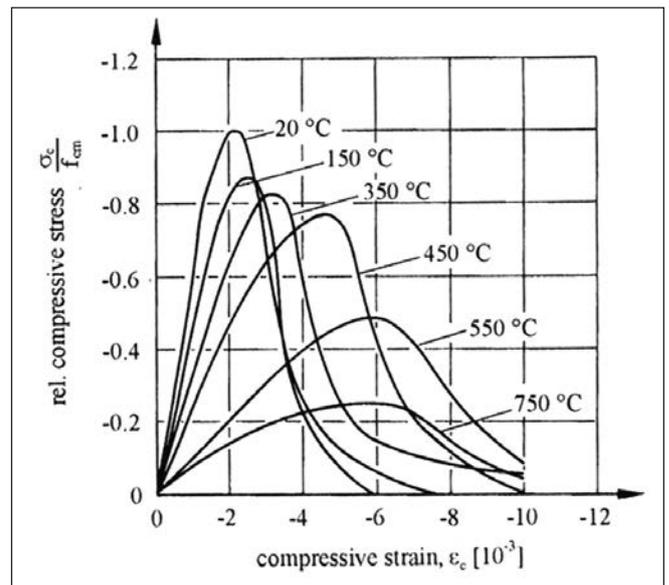
Fig. 3: Stress-strain relationship for concrete with quartz gravel aggregate as a function of temperature (Schneider, Lebeda, 2000)
