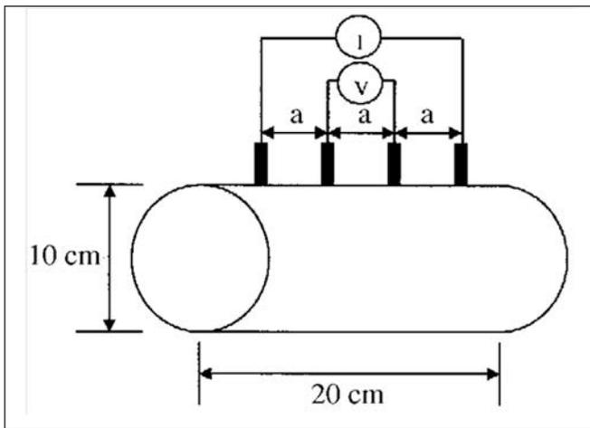
Fig. 2: The four-point Wenner probe resistivity meter
