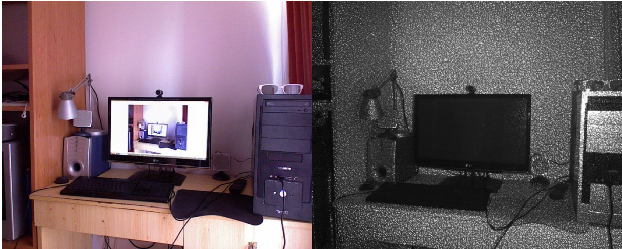
Figure 2. The color and IR images created with the Kinect
