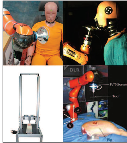
Crash tests: chest collision, neck extension, drop test device, sharp contacts with porcine leg (from top left to bottom right)
