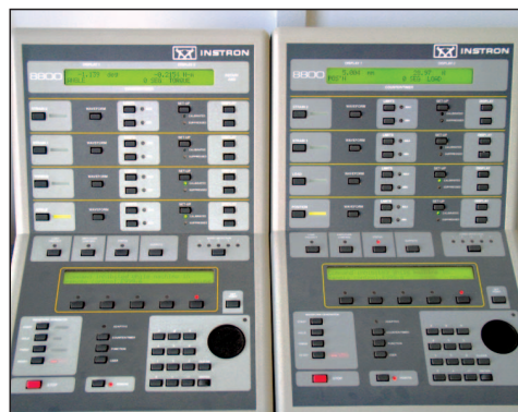
Figure 1. The consols of the Instron 8874 biomechanical material testing machine
