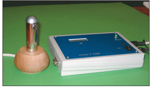
Figure 4. The finger force sensor adapter and the electronic unit
