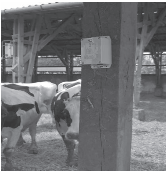
Picture 1. Temperature and humidity transponder mounted on stable wooden support
