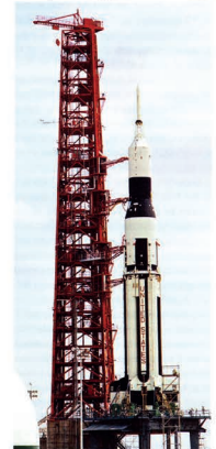
BP-13, the first Apollo boilerplate to reach orbit was launched by the Saturn I on 28 May 1964. The capsule was not recovered and burned up in the atmosphere. NASA
