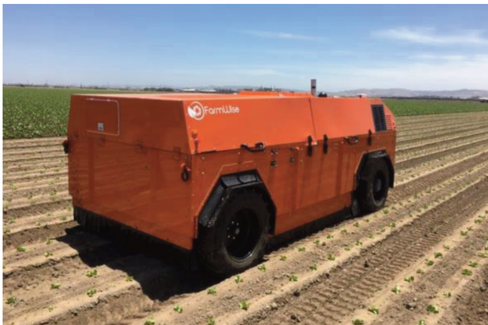
Figure 8. A robotic weeder leaves lettuce crops unharmed Source: (FarmWise,2019)
