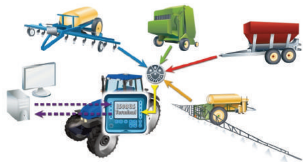
Figure 4. The data relationship between the tractor and implements with Isobus [9]
