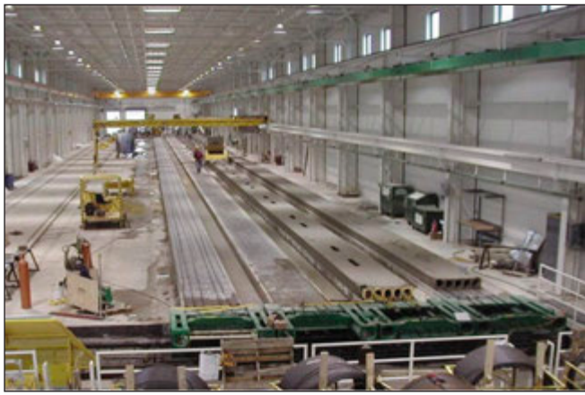
Fig. 3: Illustration for some of the steps of manufacturing HC slabs (Elematic, 2012)
