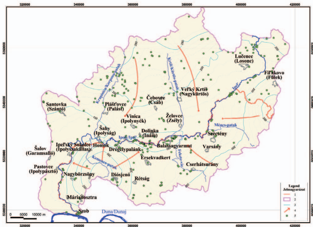
Figure 5. Calculated hydraulic potential distribution in the uppermost model-layer and the representative directions of groundwater flow, Ipoly/Ipel' Valley and its catchments model area (UTM coordinate system)
