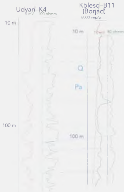
Figure 4. Correlation of Pannonian and younger beds between Udvari-K4 and Kölesd-B11 wells using well logs
