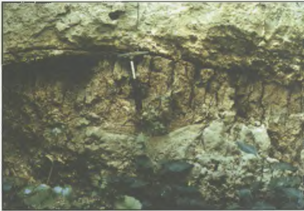
Photo 5. A detail of the outcrop 16 next to the exploratory bore-hole at Diósberény; fissured clay lens embedded in the older Pleistocene fluvial formation
