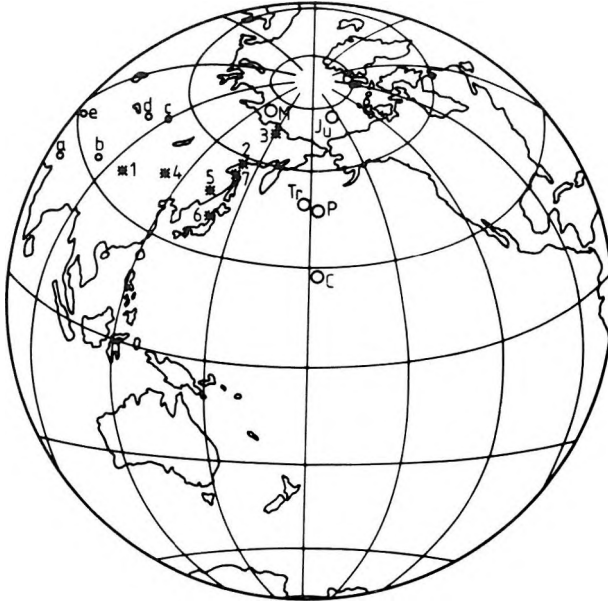
Fig. 33. Comparison between the poles in the "C" unit of Fig. 32., from areas where clockwise rotation was observed. C, P, Tr, Ju, M, a–e: for key, see Fig. 31. Palaeomagnetic poles for Greece: 1 — Epiros, Eocene; 2 — Epiros, Cretaceous; 3 — Epiros, Jurassic [HORNER 1983, HORNER and FREEMAN 1983]; 4 — Epiros, Eocene [KISSEL et al. 1985]; 5 — Chalkidiki, Eocene–Oligocene [KONDOPOULOU 1985]; 6 — for the East Carpathians, Late Cretaceous [BAZHENOV and BURTMAN 1980]; 7 — for Eastern Serbia, Late Cretaceous [STEFANOVIC and VELJOVIC 1972]
