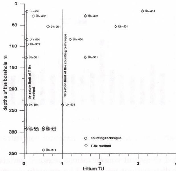
Fig. 2: Tritium contents and detection limits measured by two different techniques
