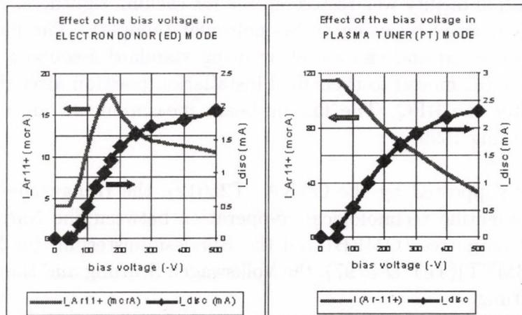
Fig. 1: The two operating modes of the auxiliary electrode in ECR ion sources
