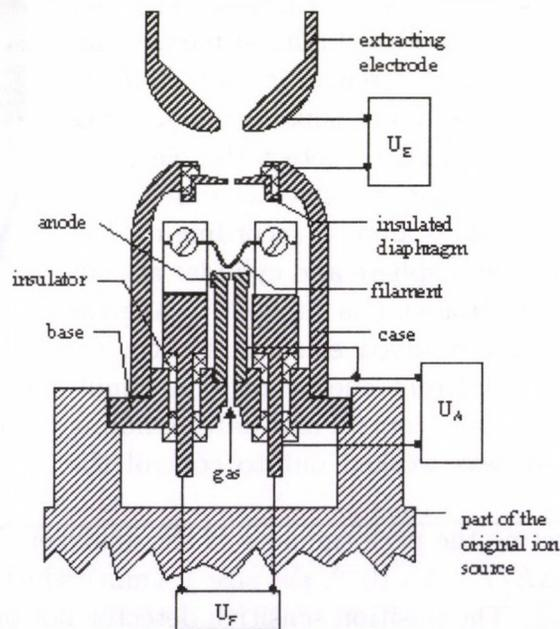
Fig. 1: The latest version of the modified ion source
