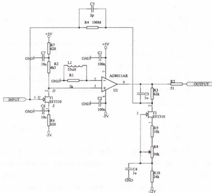
Fig. 1: Circuit diagram of the low power consumption preamplifier
