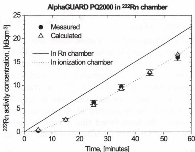
Fig. 1: Response of AlphaGUARD ionization chamber  $^{222}\text{Rn}$  monitor to linearly increasing  $^{222}\text{Rn}$  concentration. Comparison with compartment model description.
