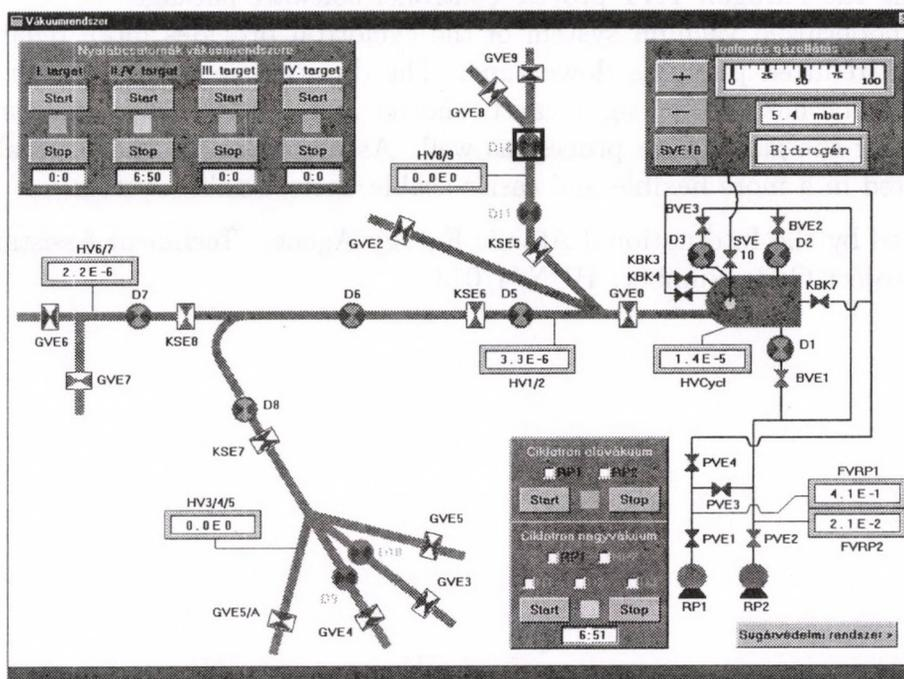
Fig. 1: The graphical user interface of the vacuum control system (the control panel text is — intentionally — in Hungarian)
