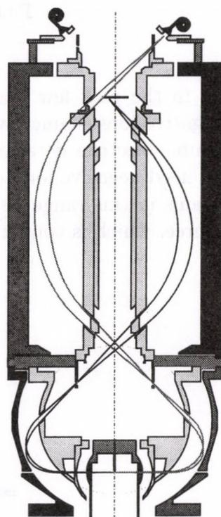
Fig. 1: The coincidence spectrometer ESA-22
