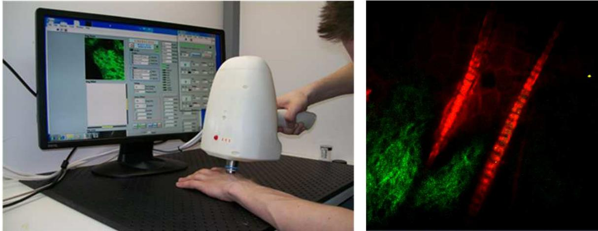
**Figure 2.** *Left:* Photo of our handhold nonlinear microscope system (FiberScope) developed for basal cell carcinoma detection. **Right:** Corresponding test image recorded for a murine skin sample at the properly set fiber laser wavelength (SHG and 2P)
