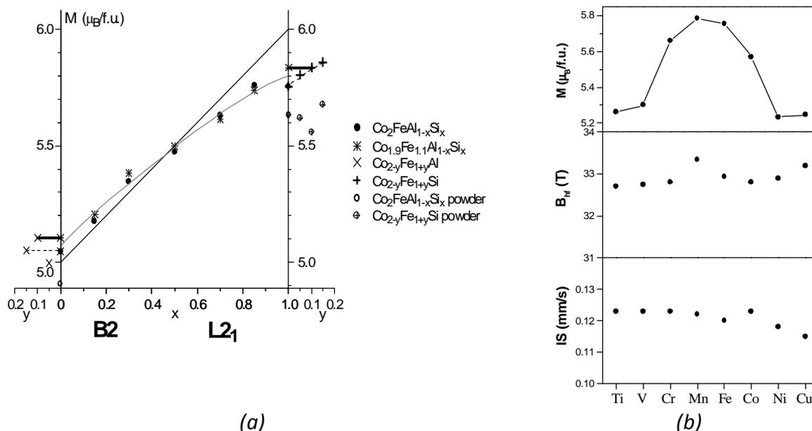
**Figure 1. a:** Average magnetization of the  $\text{Co}_2\text{Fe}(\text{Al},\text{Si})$  and related alloys. The linear composition dependence corresponds to the expected Slater-Pauling behaviour; **b:** Average magnetization, Fe hyperfine fields and isomer shifts in the  $\text{Co}_2\text{Fe}_{0.9}\text{TM}_{0.1}\text{Si}$  alloys.
