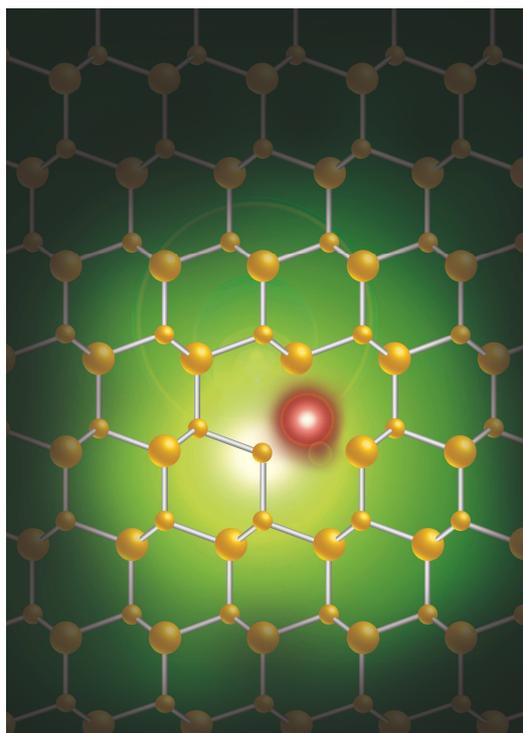
**Figure 1.** The colour centre, which emits red light, is embedded in 4H-type silicon carbide. It consists of a carbon vacancy (a carbon atom missing from SiC lattice) and a neighbouring silicon atom substituted with carbon. Silicon and carbon atoms are represented by large and small balls, respectively.
