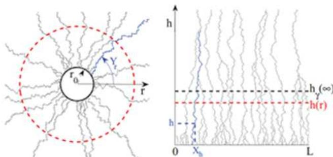
**Figure 4.** Expanding radial growth structure and the same structure on a fixed domain with periodic boundary conditions, illustrated for the case of coalescing random walks. The distribution of the rescaled radial structure at radius  $r$  is identical to the distribution of the fixed domain structure at height  $h(r)$ .
