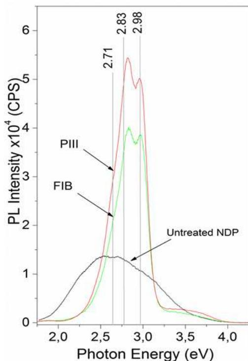
**Figure 1.** Room temperature photoluminescence spectra excited by  $E_{ex}=4.597$  eV photon energy of untreated and implanted (using PIII and FIB techniques) diamond nanocrystals after heat treatments at 750°C (in vacuum) and 450°C (in air).
