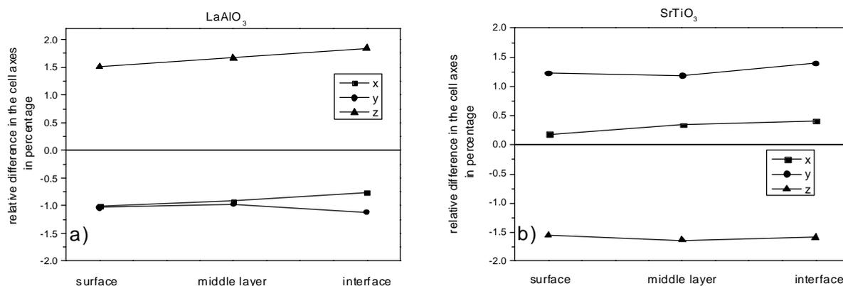
**Figure 2.** Relative differences in the cell axes of LSCO films grown on a) LaAlO<sub>3</sub> and b) SrTiO<sub>3</sub> substrates are plotted in percentage as a function of depth.
