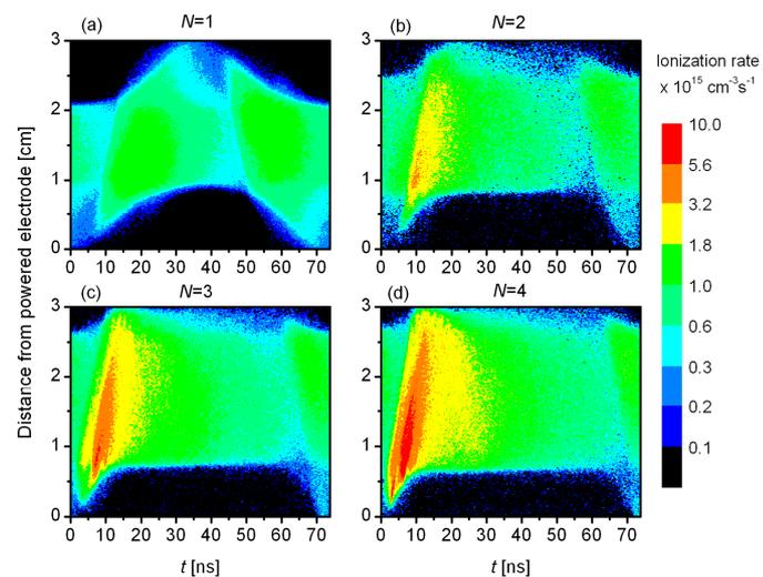
**Figure 1.** Spatio-temporal plots of the ionization rate for different number of applied harmonics,  $N$ .
