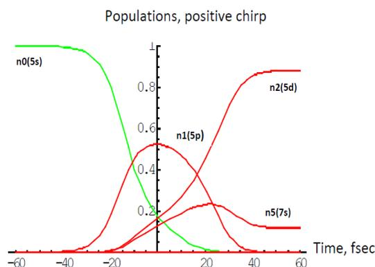
**Figure 2.** Excitation of Rb atom to states 5d and 7s by a Gaussian FC laser pulse of 30 fsec duration and positive frequency chirp. The pulse peak intensity is equal to  $3 \times 10^{12} \text{ W/cm}^2$ , the speed of the linear chirp is  $0.3 \text{ fs}^{-2}$ .
