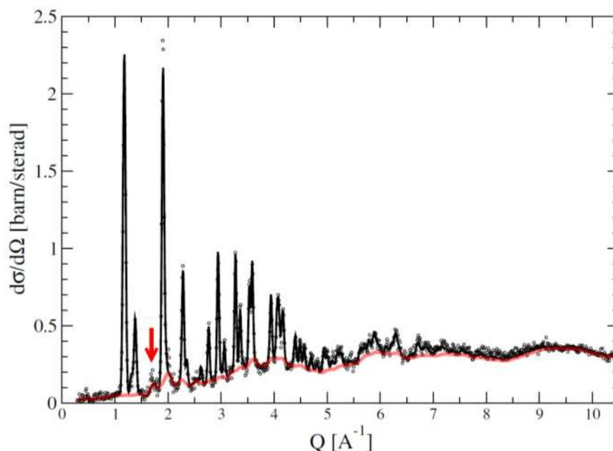
**Figure 5.** Experimental and simulated neutron powder diffraction patterns of tetragonal  $Cl_4$ . Circles: measured differential cross section; black solid line: RMCPOW; red solid line: the separated diffuse contribution. The red arrow indicates the strongest parasitic Bragg-peak, most probably from iodine.
