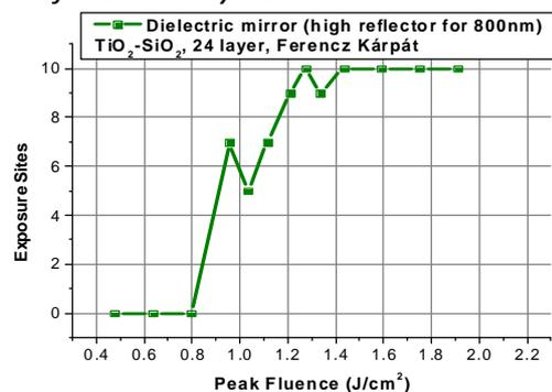
*Damage threshold of laser mirrors*
