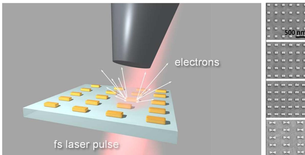
**Figure 1.** Experimental scheme on photoemission from metallic nanoparticles, including nanorods on a glass substrate. The illuminating femtosecond laser beam comes from below and the spectrometer tube collecting the electrons is also depicted. The different nanoparticles investigated are shown on the right-hand-side.
