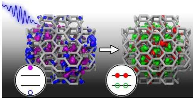
**Figure 5.** BC8 body-centered cubic silicon nanocrystal. A high-energy (blue) photon produces a high-energy electron-hole pair, which very efficiently decays to two pairs of lower energy holes and electrons thereafter. Distributions of probabilities of finding the electrons and holes are shown with clouds of their respective schematic colours.
