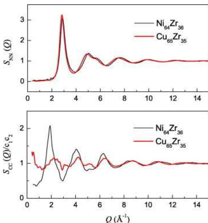
**Figure 1.** Comparison of the Bhatia-Thornton number-number (**upper panel**) and composition-composition (**lower panel**) partial structure factors of  $Ni_{64}Zr_{36}$  and  $Cu_{65}Zr_{35}$ .
