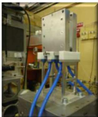
**Figure 2.** The new biomembrane option for the GINA neutron reflectometer
