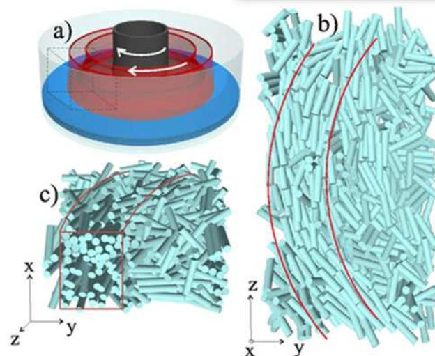
**Figure 1.** Shear induced ordering of elongated particles. Image (a) shows the experimental split bottom shear cell, while images (b) and (c) show the reconstructed particle positions and orientations from the tomographic images.
