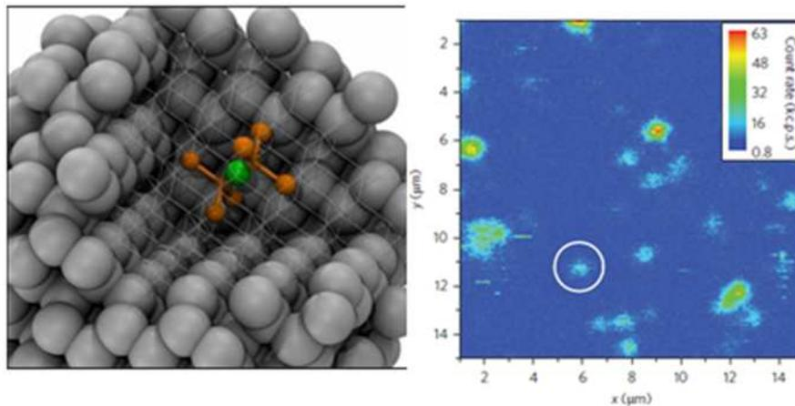
**Figure 2.** The molecule-sized nanodiamond and the embedded SiV colour centre (a pair formed from a substitutional silicon atom and a vacancy). The spots in the false-colour confocal microscope image shows the locations of such nanodiamonds, red middle regions correspond to brighter areas.
