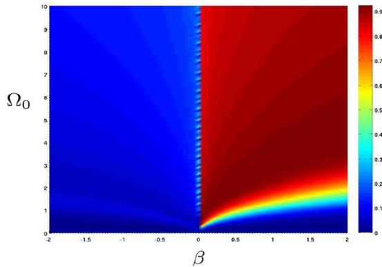
**Figure 3.** Dependence of the final population of the state 5d of the Rb atom on peak Rabi frequency  $\Omega_0$  of the laser pulse (in units of  $\text{fsec}^{-1}$ ) and chirp speed  $\beta$  (in the units of  $\text{fsec}^{-2}$ ).
