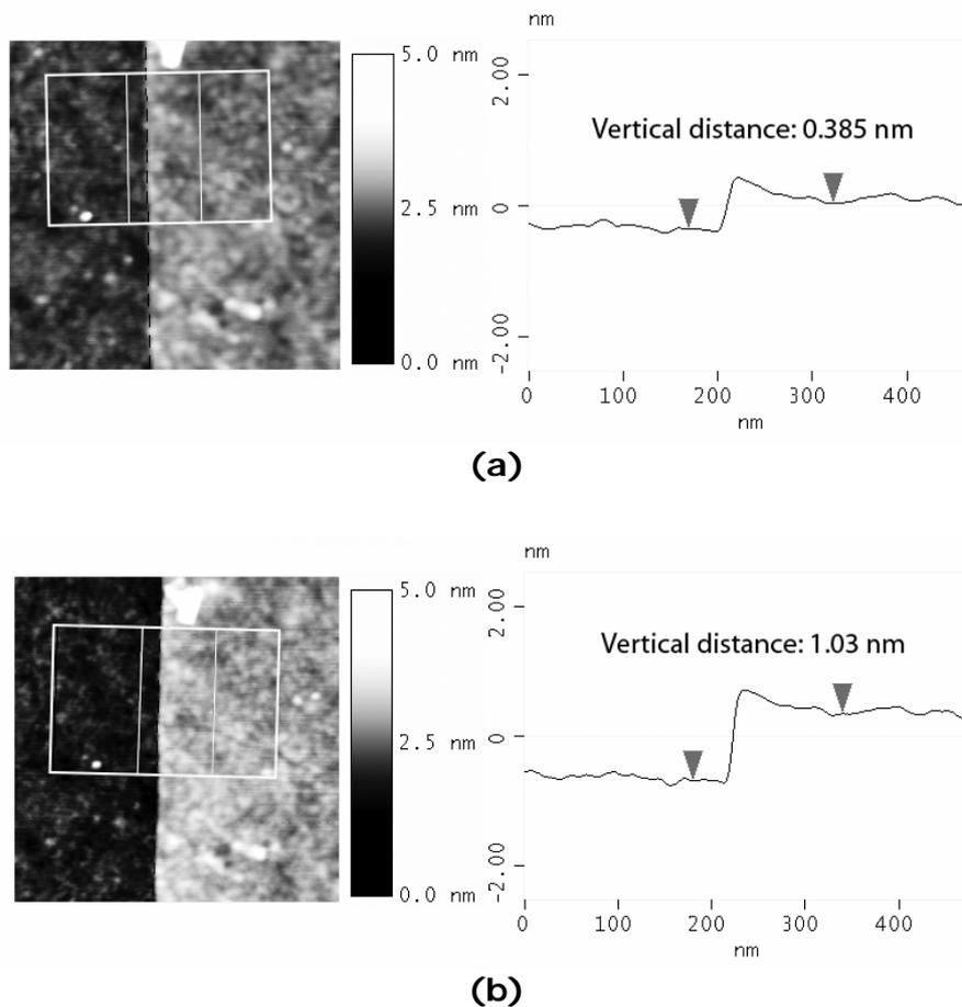
**Figure 4.** Two consecutive measurements *on the same graphene layer*, with differing free amplitude of the cantilever. a.) 150 mV, b.) 65 mV At the higher free amplitude setting the measured thickness increases significantly. (see linecut)
