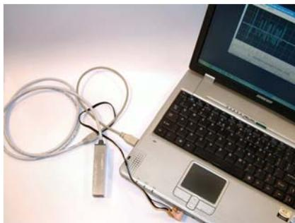
**Figure 2** Fluxset measuring probe connected with laptop for reading out of logistic bars. Signals from the barcodes and result of decoding are seen on the screen.
