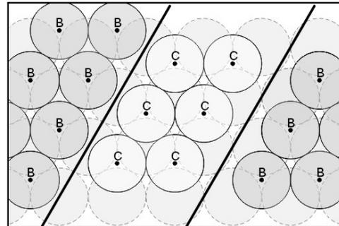
**Figure 5** Phase-boundaries that can be formed on the triangular fcc surface.
