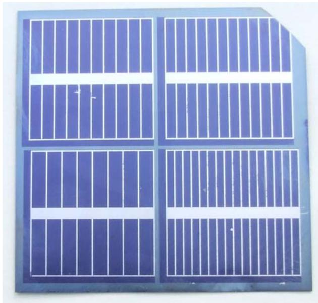
**Figure 15** The photograph of ultra shallow emitter solar cells with different metallization grids on  $5 \times 5 \text{ cm}^2$  Si wafer. In order to obtain optimal serial resistance for the PIII cells, 4 different metal grids were tested. These metal grids are applicable in a wide range of emitter resistance (90-300 Ohm/sq).
