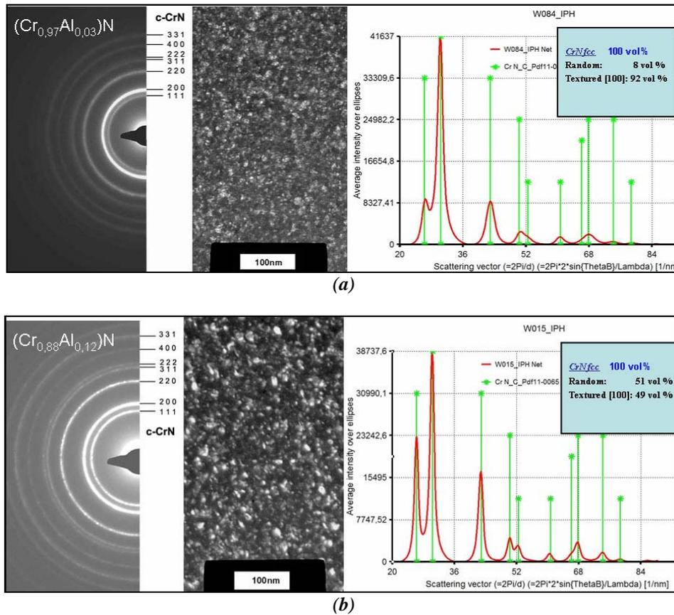
**Figure. 17** SAED patterns, DF TEM images and the ProcessDiffraction evaluation of the SAED patterns. The volume fraction of the fcc and hcp phases as well as the textures are given
