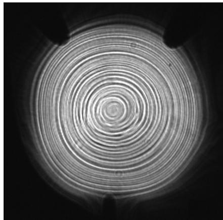
**Figure 5** Makyoh-topography image of a *p*-type Si wafer having swirl defect
