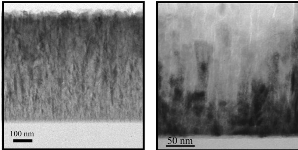
**Figure 13** The structure of C-Ti (right) and C-Ni (left) samples prepared at 200 °C
