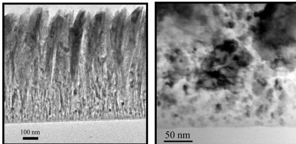
**Figure 14** The structure of C-Ti (right) and C-Ni (left) samples prepared at 800 °C.
