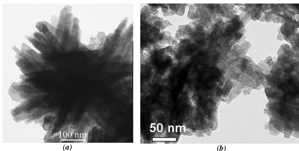
**Figure 4** TEM images of tungsten oxide nanopowder. (a) orthorhombic „mother” phase of  $\text{WO}_3 \cdot 1/3\text{H}_2\text{O}$ , (b) hexagonal  $\text{WO}_3$ .
