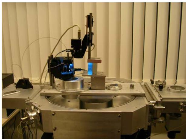
*Figure 3* Photograph of the new version of the wide-angle ellipsometer (equipped with a spherical mirror) mounted to the diagnostic chamber of a metal organic chemical vapor deposition system.
