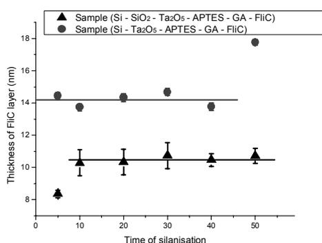
**Figure 1** Thickness of FliC (immobilized protein) layer as the function of silanization time. Average thickness is shown by the thick lines (excluding the two outliers). Samples with the native oxide (●) and with the thermal oxide (▲) are presented.
