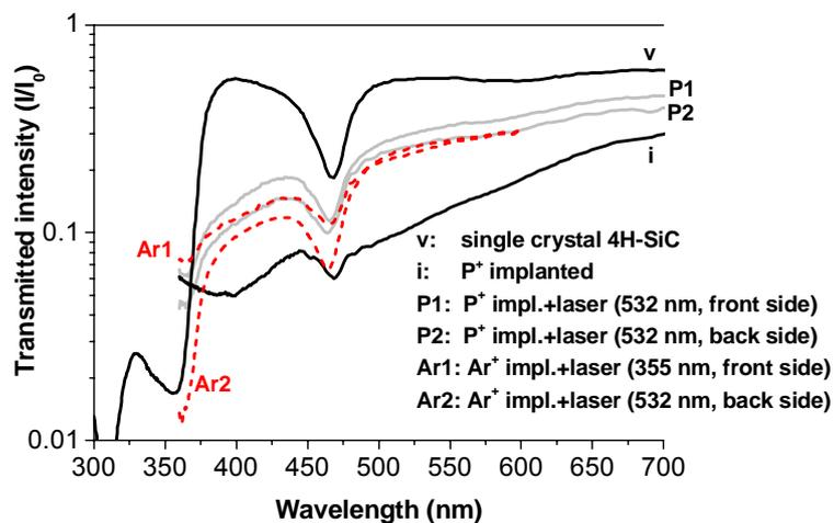
**Figure 13** Optical transmission measured on double side polished 4H-SiC samples with thickness of 400  $\mu\text{m}$ . Data for single crystalline, as-implanted, and post-implantation laser annealed samples are also shown.
