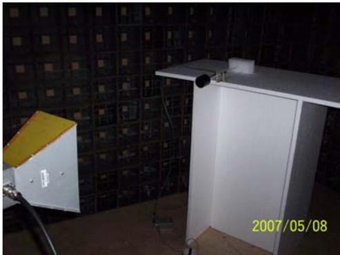
**Figure 18** The calibration of the probe in anechoic chamber with the calibrated horn antenna.
