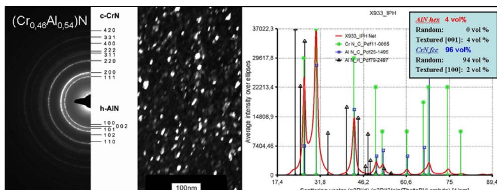
Figure 18 At 54 at% Al the hexagonal phase is well detected
