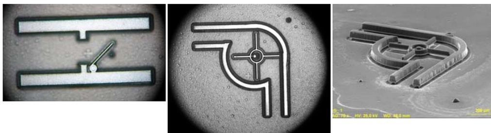
**Figure 7** Microfluidic valve (left) and turbine (middle & right) realized by proton direct writing and porous Si etching
