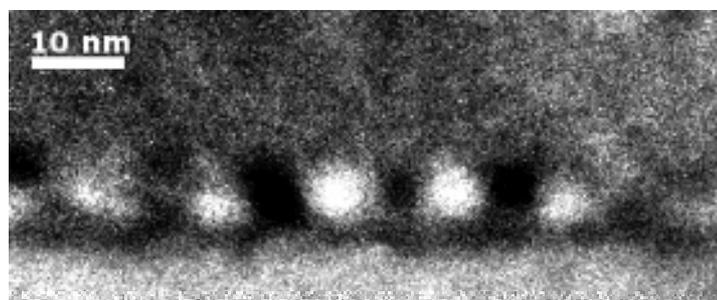
**Figure 10** Energy-filtered XTEM image of sample No. 1 with white dots corresponding to silicon atoms – spherical objects in the middle of the figure are corresponding to the Si NCs embedded between two Si<sub>3</sub>N<sub>4</sub> layers.
