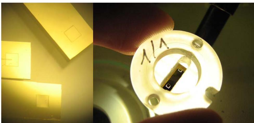
*Figure 6 The manufactured micro-cantilever structures (left) and a packaged device (right).*
