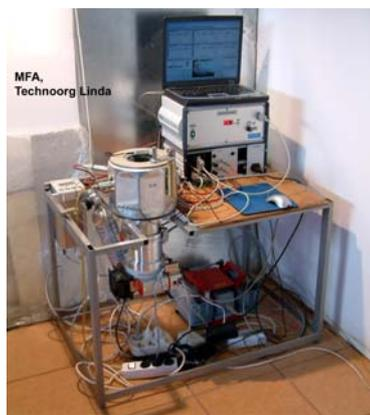
**Figure 27** Test chamber with the 20 keV ion gun.
