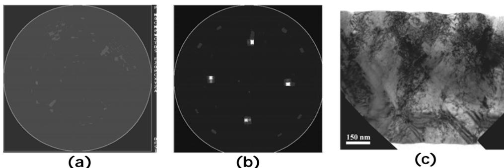
**Figure 10**  $\langle 111 \rangle$  pole figures of Cu films of 50 nm thickness (a), 400 nm thickness (b) and TEM bright field cross section image of the 400 nm thick film (c).
