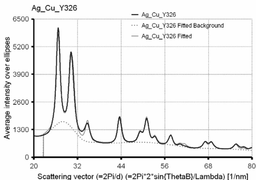
**Figure 1:** Example of the measured and the fitted distributions. Sample: sequentially evaporated 10 nm Ag and 10 nm Cu on a self-supporting substrate of 5 nm amorphous-Carbon. Analysis result is 51 vol% Ag / 49 vol% Cu
