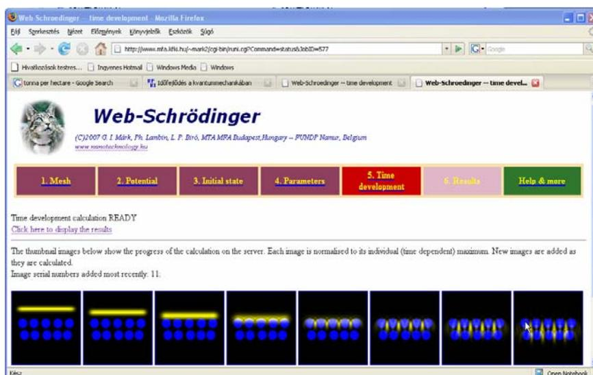
**Figure 8** Interactive wave packet dynamical simulation of the transport of an electronic wave packet through a quasi ordered nanosystem
