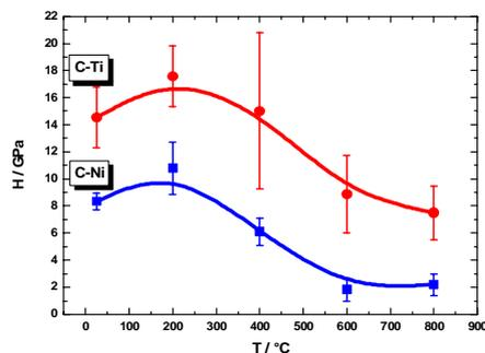
**Figure 15** The hardness of the nanocomposite thin films as the function of deposition temperature
