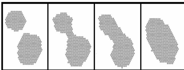
**Figure 7** Observed island coalescence scenario in simulations. Simulation parameters are:  $T=450\text{ K}$  and  $F=0.1\text{ ML/s}$ .
