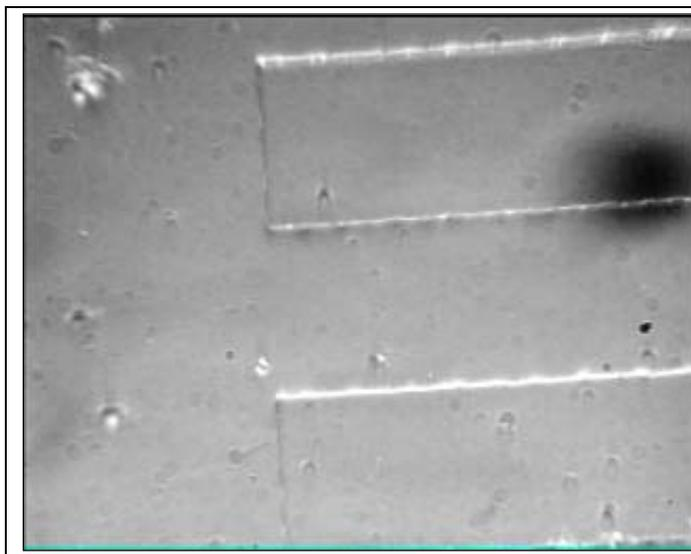
*Figure 7 The pattern of a 4  $\mu\text{m}$  thick SiON layer.*
