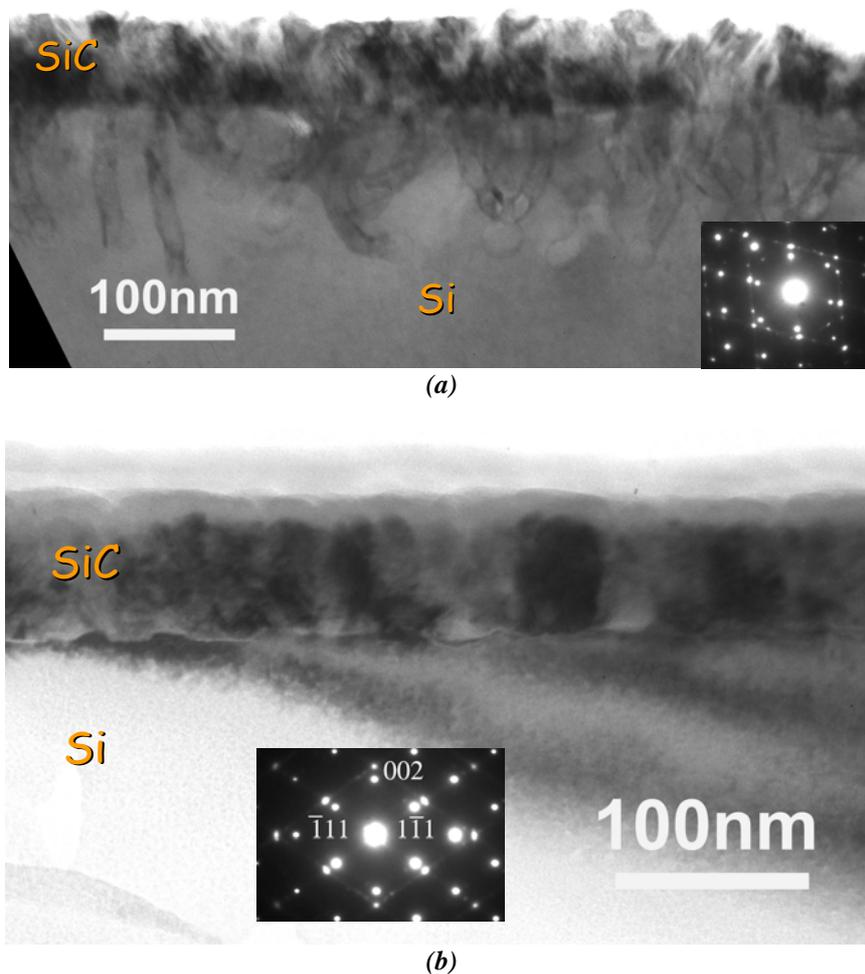
**Figure 9** Cross sectional transmission electron microscopy image of CVD deposited 3C-SiC layers on (100) Si, (a) conventional method with carbonization step, wormholes are formed during the CVD deposition, (b) SiC nanocrystals formed by CO reactive annealing were used before the CVD step, no void or wormhole formation is present.
