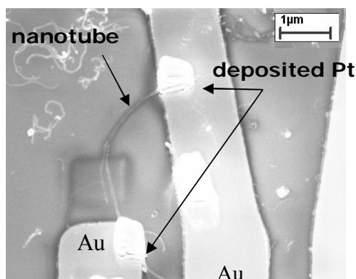
**Figure 2** Individual CNT contacted to gold electrodes by electron beam assisted Pt deposition
