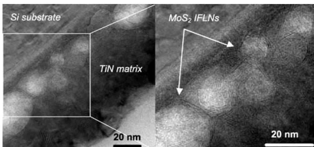
**Figure 3** (Left) Cross section TEM micrograph of a MoS<sub>2</sub>/TiN nanocomposite film produced using the multilayer deposition mode. 10–50 nm size IFLN-MoS<sub>2</sub> are dispersed in the TiN matrix. The silicon substrate and TiN matrix can be clearly recognized. (Right) higher magnification view of the same region showing the structure of MoS<sub>2</sub> nanoparticles.
