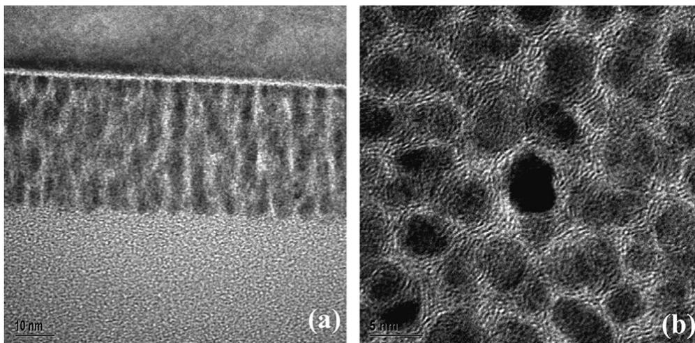
**Figure 2** Cross-sectional (a) and plan-view (b) high-resolution TEM images of the C:Ni composite thin film grown at 300 °C.
