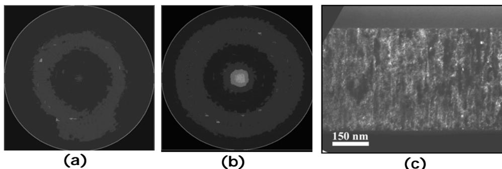
**Figure 12.**  $\langle 111 \rangle$  pole figures of Cu-Ag films of eutectic composition of 50 nm thickness (a), 400 nm thickness (b) and TEM dark field cross section image of the 400 nm thick film (c).
