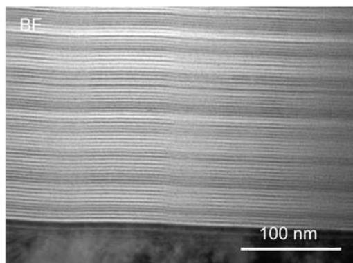
**Figure 22.** Cross sectional electron micrograph of the multilayer coating CrC/graphite
