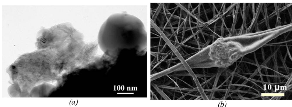
**Figure 3** Nanocrystalline bi-modal hydroxyapatite from eggshell (a) and fibrous structure of hydroxyapatite-polymer composite (b) [15].
