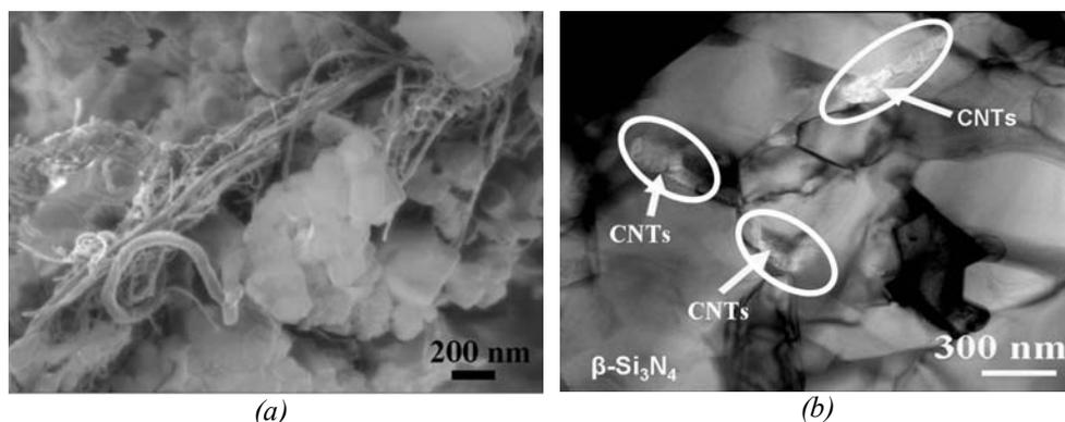
**Figure 1** Structure of  $\text{Si}_3\text{N}_4$  based nanocomposite with carbon nanotube addition. (a) SEM image of starting powder mixture before sintering, (b) TEM image of sintered nanocomposite [12].
