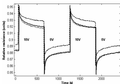
**Figure 1.** Relative resistance versus time plot of a mat of CNTs with 0.6% ethanol (continuous), 3% ethanol (dashed), and 2.4% acetone (dotted line) v/v in air concentration, changing the gate voltage (value displayed in the middle)
