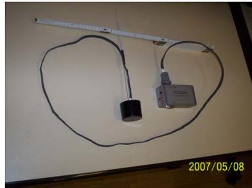
**Figure 19** The isotropic E-field probe with the flexible leads.
