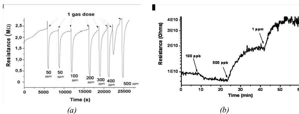
**Figure 5** Sensing properties of  $h\text{-WO}_3$  to  $\text{NH}_3$  at  $300^\circ\text{C}$  (a) and  $\text{NO}_2$  at  $150^\circ\text{C}$  (b).
