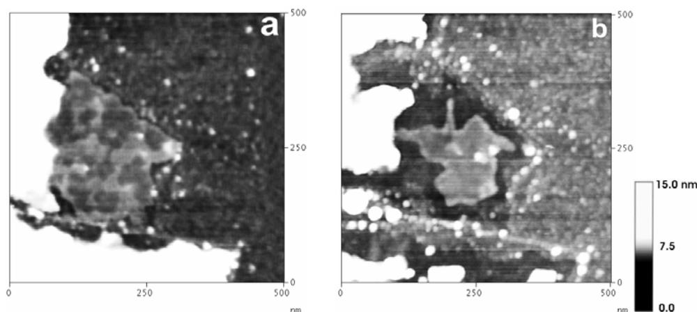
**Figure 3** Tapping mode AFM images ( $500 \times 500 \text{ nm}^2$ ) showing the effect of oxidation. The images were recorded after oxidation step II (a) and after oxidation step III (b). A lacy, incomplete top layer can be observed in (a), whereas a single atomic layer was left behind in (b).
