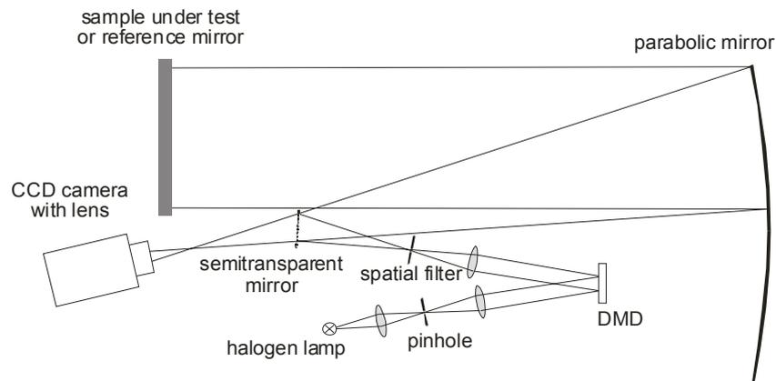
**Figure 4** Layout of the Makyoh-topography set-up with the DMD
