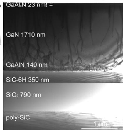
**Figure 21** Typical nitride layers grown onto the thin hexagonal SiC strip of the hybrid substrate. Threading dislocations are well visible.
