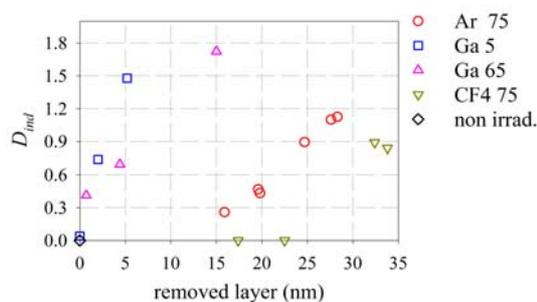
**Figure 24** The broadening of the interface vs removed layer thickness due to ion irradiation of various projectiles of 20 keV. 5 and 65 in the caption stands for irradiation applying angles of 5 and  $65^\circ$ .  $D_{ind}$  is the parameter of the logistic function fitting the transition.
