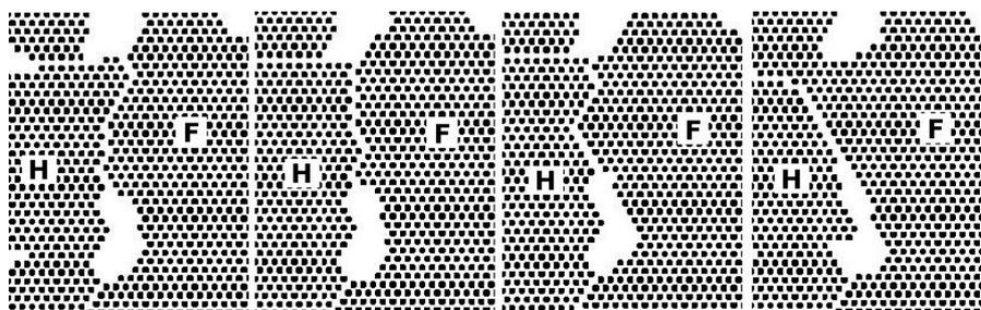
**Figure 6** Characteristic time evolution and annihilation of stacking faults related phase-boundaries for the case when only A type of atoms are deposited. The pictures from left to right represent some steps in the time-evolution. The F and H islands correspond to fcc and hcp stacking, respectively. Simulation parameters are:  $E_{AA}=0.15\text{eV}$ ,  $T=650\text{K}$ ,  $F=10\text{ML/s}$  and  $f_0=10^{12}\text{ Hz}$ .
