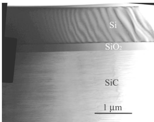
**Figure 20** Thin Si layers transferred onto polycrystalline SiC substrate by smart-cut technique with a surface roughness of rms < 1 nm.
