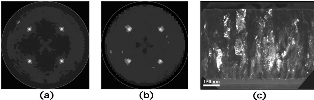
**Figure 11**  $\langle 111 \rangle$  pole figures of Cu 10 at%Ag films of 50 nm thickness (a), 400 nm thickness (b) and TEM dark field cross section image of the 400 nm thick film (c).
