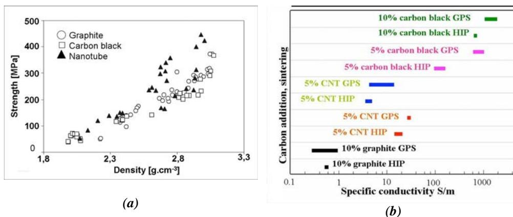
**Figure 2** Mechanical (a) and electrical (b) properties of  $\text{Si}_3\text{N}_4$  based nanocomposites with different carbon addition.
