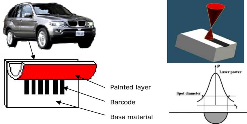
**Figure 1** Laser marking. Invisible car identification and process of laser scribing
