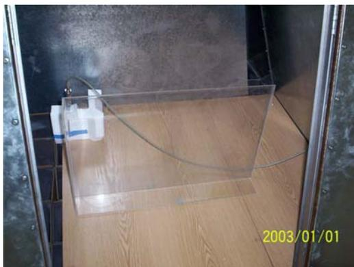
**Figure 17** The measuring set-up for the field scattering effect. In the photo the field distribution of the plexiglass sheet is investigated in the GTEM cell.
