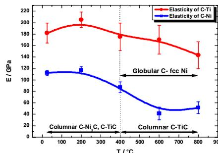
**Figure 16** The modulus of elasticity of the nanocomposite thin films as the function of deposition temperature
