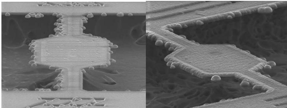
*Figure 8 Poly-silicon micro-heater formed by diamond SAD technique.*
