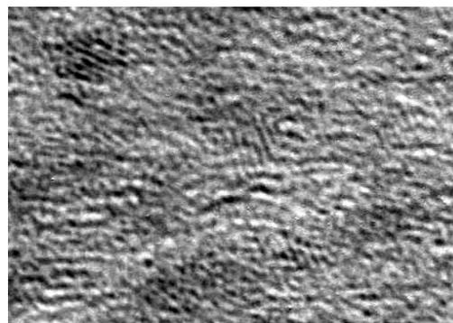
**Figure 23.** Both (111) and (002) lattice planes of the fcc CrC phase as well as the (0002) spacing of the randomly oriented graphite phase were observed on the high resolution electron micrograph.
