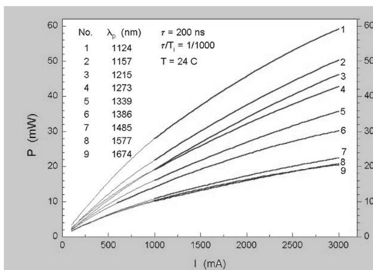
*Figure 16* Output power of the different wavelength LED's as a function of pulse current
