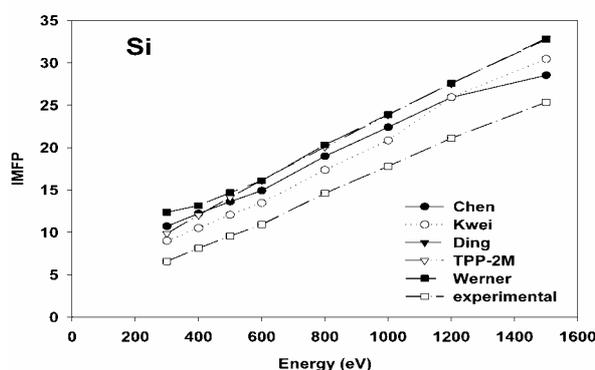
*Figure 25 Comparison of the uncorrected IMFPs with the SEP corrected curves of Si. Best approach was achieved with material parameters of Chen (improved) and Werner*
