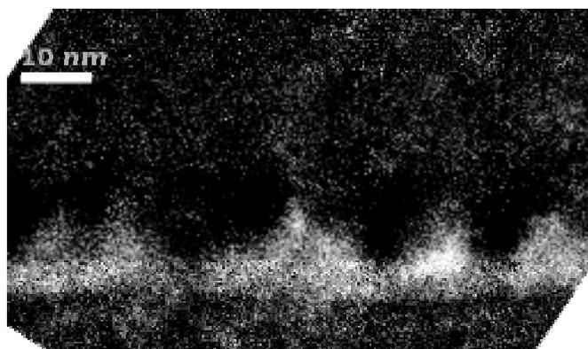
**Figure 11** Energy-filtered XTEM image of sample No. 2 with white dots corresponding to oxygen atoms – image indicates SiO<sub>2</sub> pyramids between the Si NCs.
