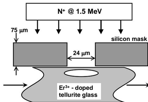
**Figure 2** Sketch of the setup used to fabricate channel waveguides in  $\text{Er}^{3+}$ -doped tellurite glass by ion irradiation. A silicon mask, with an opening of about  $24\ \mu\text{m}$ , is placed in front of the sample before each exposure in order to define a channel waveguide.
