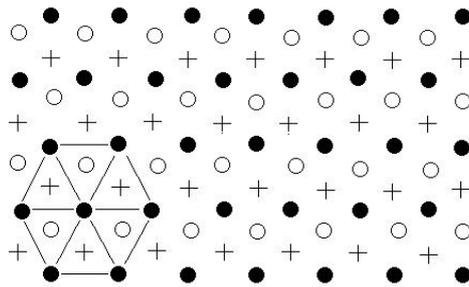
**Figure 4** Geometry of the considered lattice. Filled circles represent the sites of the substrate, empty circles and crosses represent the fcc and hcp lattice sites, respectively, on which the new layer can grow
