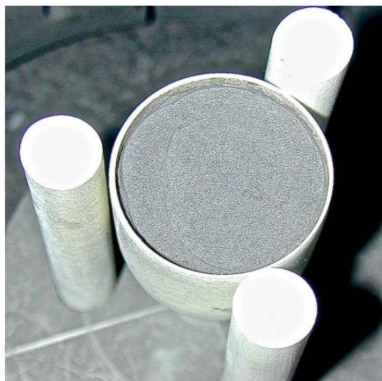
Figure 1. Crucible and its support before the melting runs.
