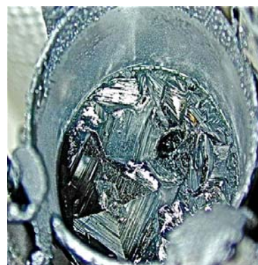
Figure 5. Most perfect polycrystalline sample grown (a) after and (b) before being removed from the crucible.
