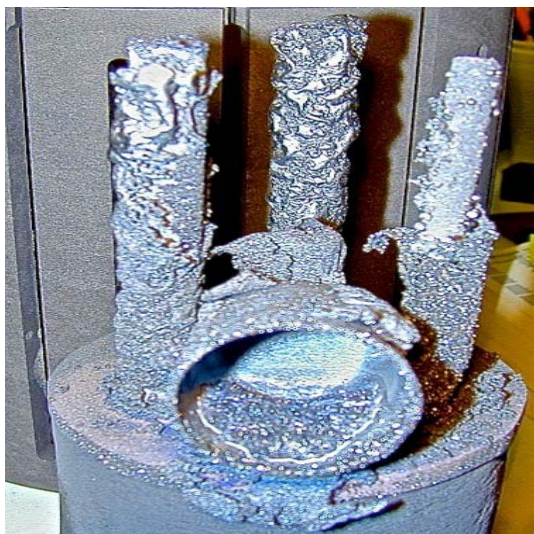
Figure 4. When erosion of rods is very intensive, they are unable to support the crucible.
