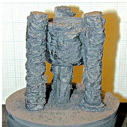
Figure 3. Rods and crucible entirely covered with silicon-colored deposit.
