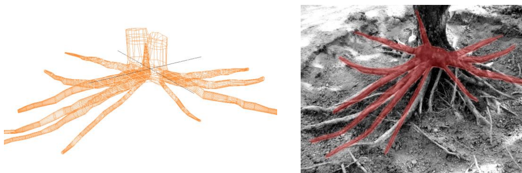
Figure 5. The 3D model of the root system (left) compared to the result of excavation (right) (Divós et al. 2009)
