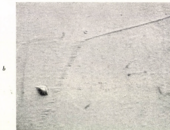
Fig. 5. Etch figures observed on polished prism surfaces. a) The solution of the polished surface begins at places, where the lattice has been deformed. Etch figure originated by deformation caused by the rawer grains of the polishing material. b) Small angle boundaries with a dislocation density of 10^4 \text{ cm}^{-1}
