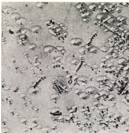
Fig. 2. Next to the smaller hillocks etch pits become visible. To every hillock belongs an etch pit. 100 ×
